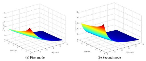
Fig. 8 The effects of span length and the number of span on frequencies of the plain concrete arch bridges. (a) the first mode, and (b) the second mode
