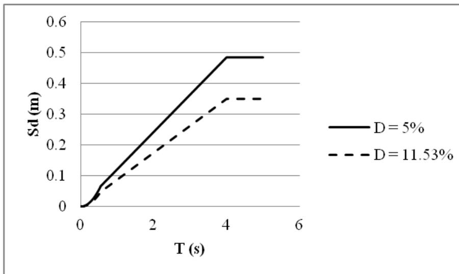
Fig. 6 Displacement response spectra
