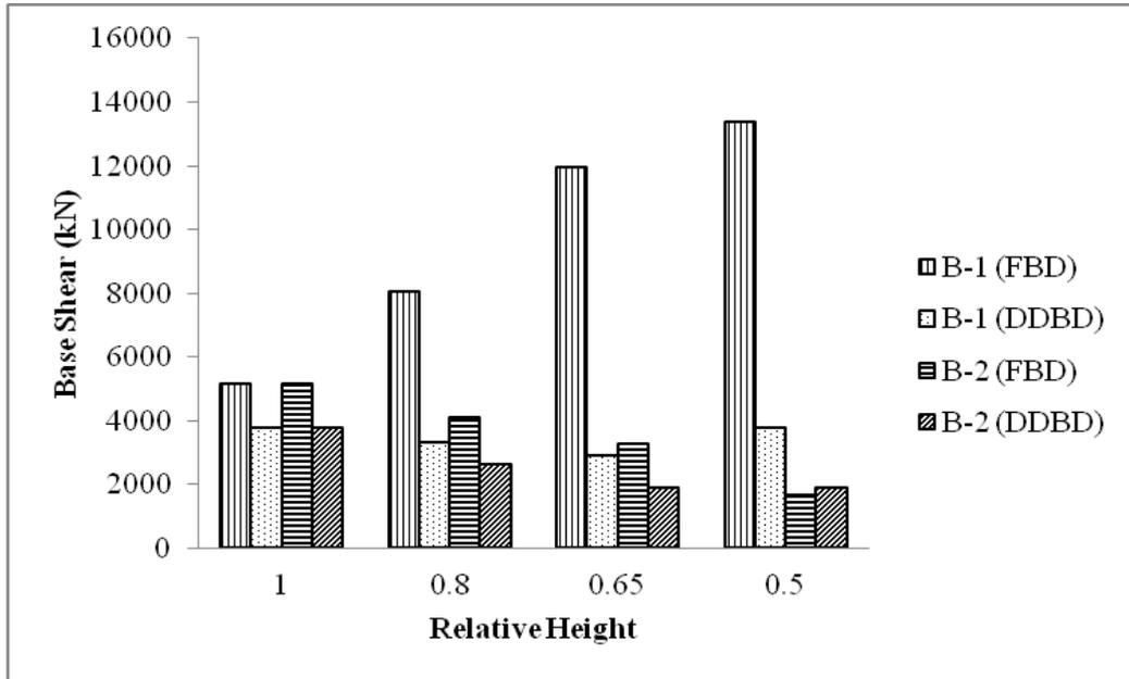
Fig. 7 Variation of base shear at bents with design methodology
