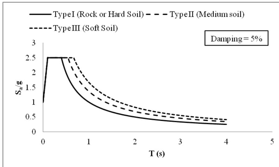
Fig. 5 Response spectrum as per IRC 6 (2010)
