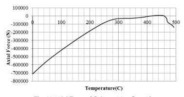
Fig. 11 Axial Force of Column A1 at floor 10
