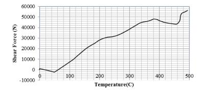
Fig. 7 Shear Force of Beam B1A1 at floor 10
