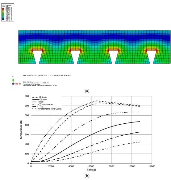
Fig. 4 Heat transferring result of slab and parametric fire temperature curve
