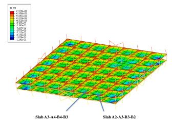
Fig. 19 Contour of Vertical deformation of slabs on floor 9, 10
