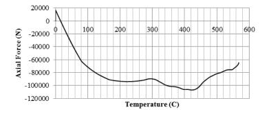
Fig. 24 Axial Force at the perimeter of slab A2-A3-B3-B2 at floor 10
