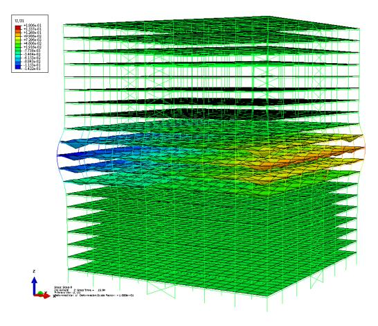
Fig. 10 Horizontal deflection of the model (deformation is amplified)
