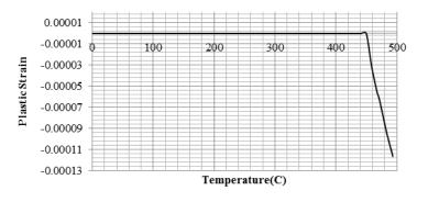
Fig. 18 Plastic strain in Brace on Grid D1 at floor 10
