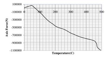
Fig. 6 Axial Force of Beam B1A1 at floor 10
