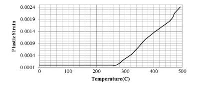
Fig. 14 Plastic strain in Column A1 at floor 10
