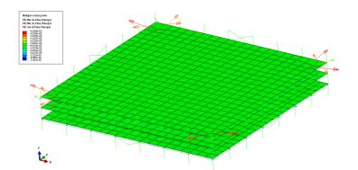
Fig. 20 Crack pattern (tensor of plastic strain) of the concrete slab on floor 9, 10 and 11
