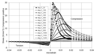
Fig. 3 Stress- Strain relationship of Concrete by EN1994-1-2 (2005)
