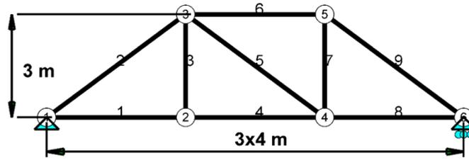
Fig. 1 Nine bar truss
