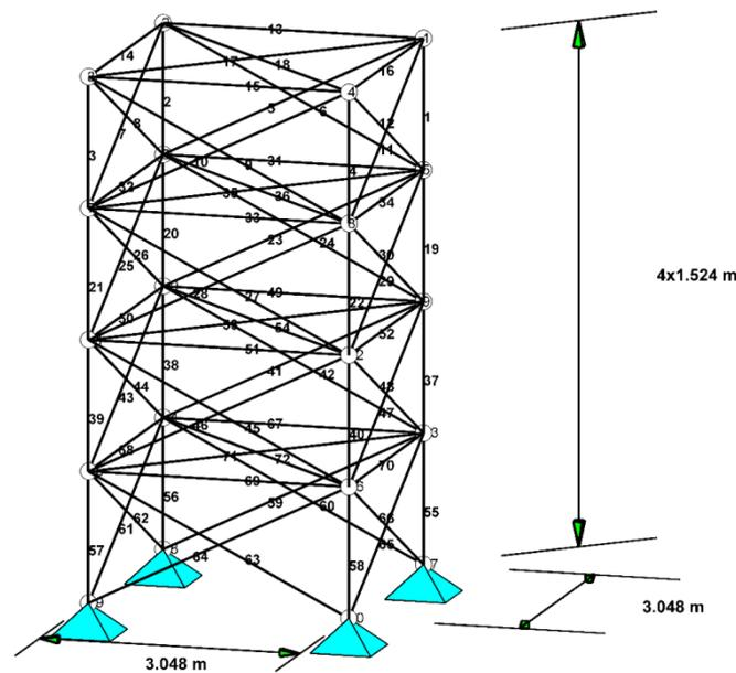
Fig. 3 Seventy-two bar truss
