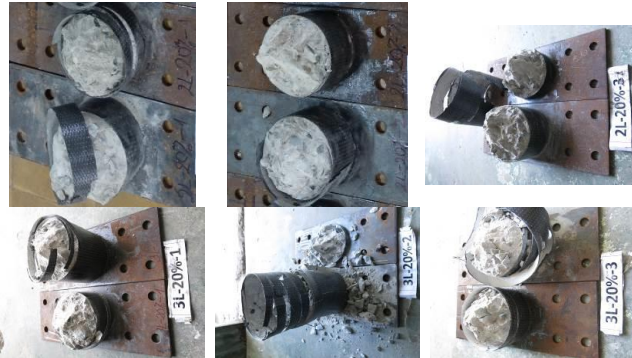
(b) Specimens with preload 20%
