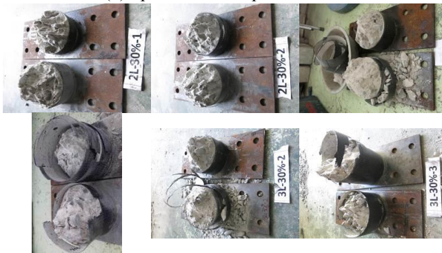
(c) Specimens with preload 30%
