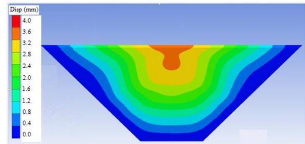
Fig. 10 (b) Displacement contour diagram of the body under blasting analysis
