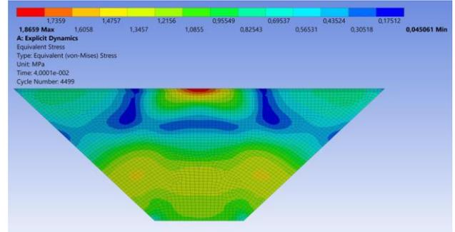
Fig. 12 (a) Stress contour diagram of the body under hydrostatic analysis
