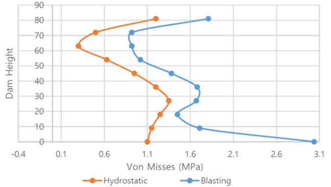
Fig. 13 (a) Von Mises Stress changes through dam height
