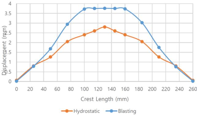
Fig. 11 (b) Maximum displacement changes through crest length
