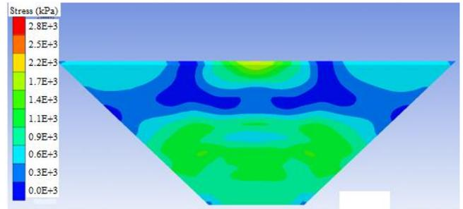
Fig. 12 (b) Stress contour diagram of the body under blasting analysis
