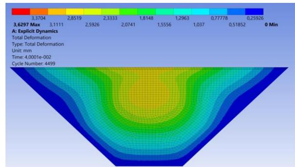
Fig. 10 (a) Displacement contour diagram of the body under hydrostatic analysis
