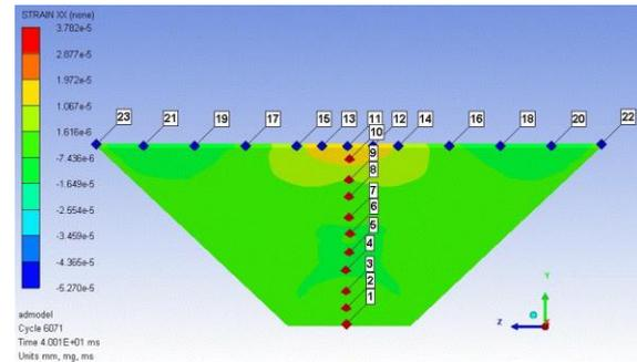
Fig. 14 (b) Strain contour diagram of the body under blasting analysis
