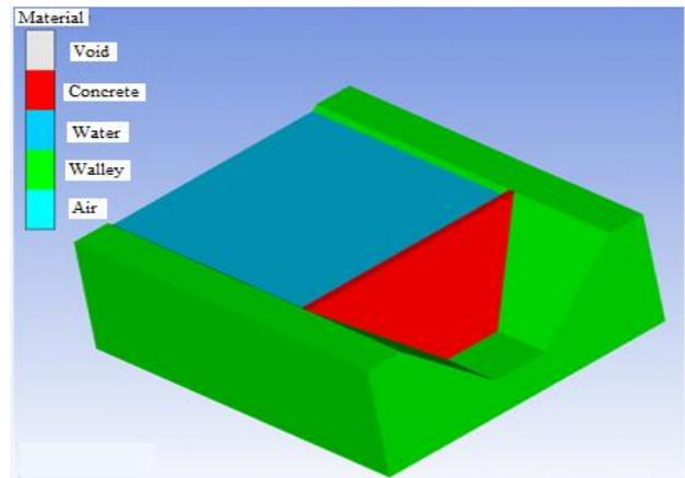
Fig. 4 3D finite element model of Sariyar gravity dam
