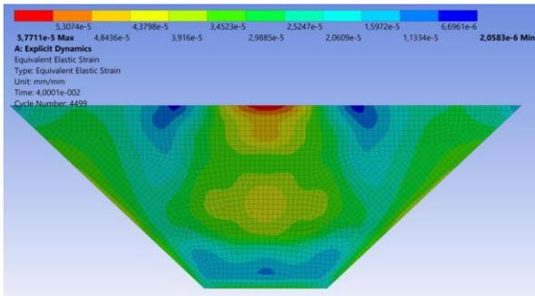
Fig. 14 (a) Strain contour diagram of the body under hydrostatic analysis
