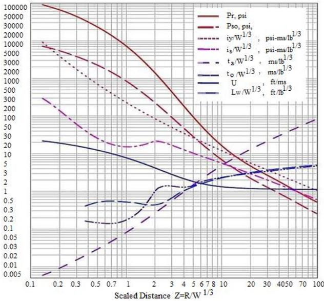
Fig. 2 Parameters of positive phase of TNT charges from free-air bursts (UFC 3- 340-02 2008)
