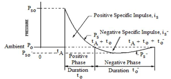
Fig. 1 Time histories of pressures due to explosions (UFC 3-340-02 2008)
