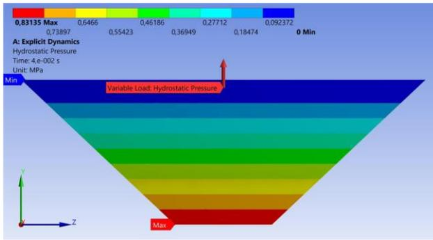
Fig. 5 Applied hydrostatic pressure on the side of the gravity dam
