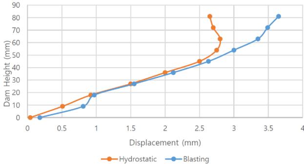
Fig. 11 (a) Maximum displacement changes through dam height
