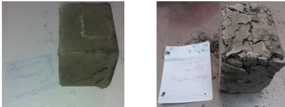
(a) With lower steel fiber ratio and inside large cracks (b) With higher steel fiber ratio and surficial cracks
