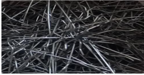
Fig. 2 Used hooked steel fibers in concrete mix design
