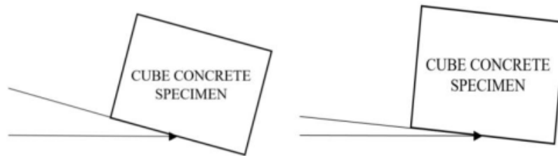
Fig. 4 Different impact angels used for abrasion evaluation
