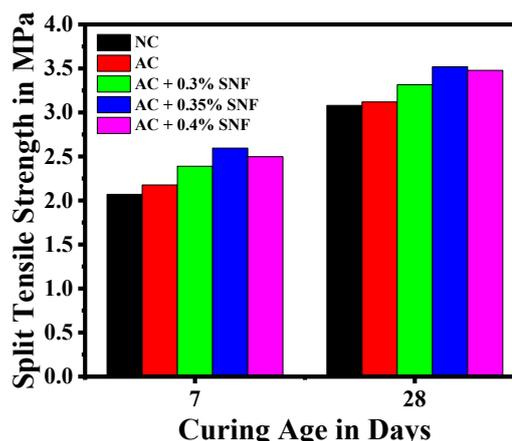
Fig. 4 Split tensile strength variation of concrete mixes
