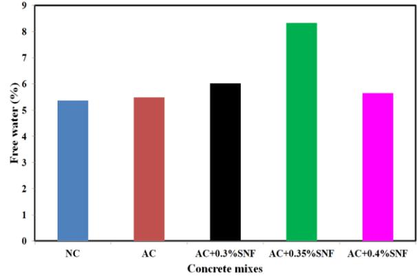
Fig. 10 Free water (%) of different concrete mixes
