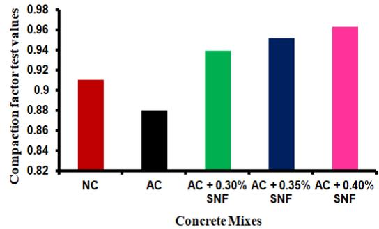
Fig. 2 Compaction factor values with different mixes
