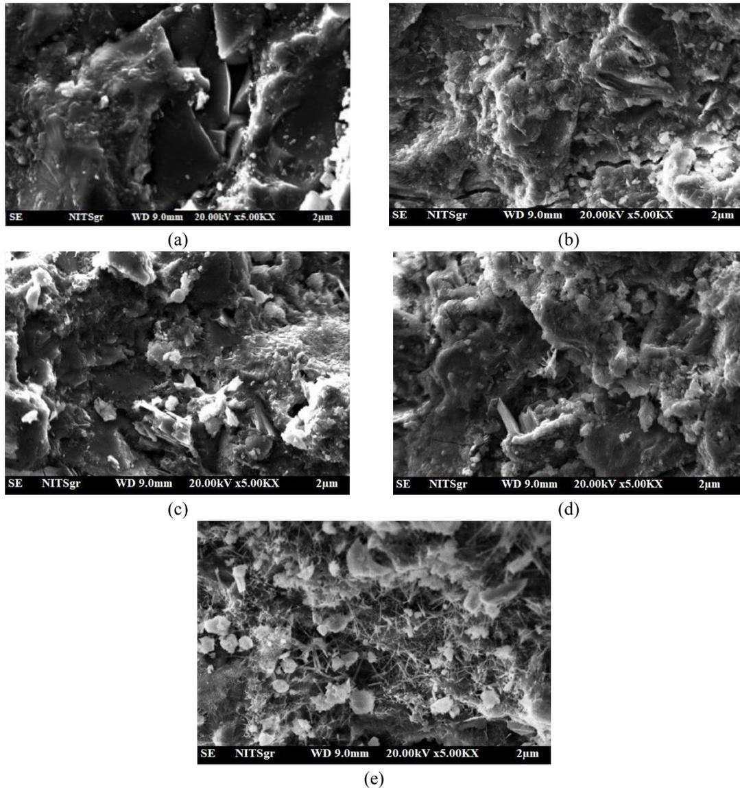
Fig. 13 SEM analysis of (a) Normal concrete, (b) Alccofine concrete, (c) Alccofine + 0.30% SNF (d) Alccofine + 0.35% SNF and (e) Alccofine + 0.40% SNF
