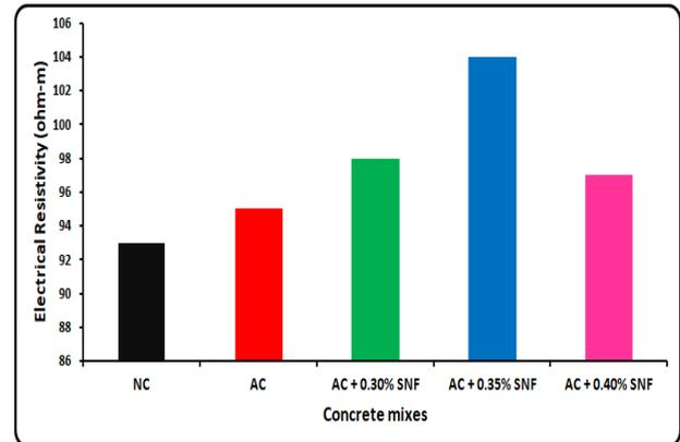
Fig. 7 Graphical representation of electrical resistivity of early strength concrete mixes
