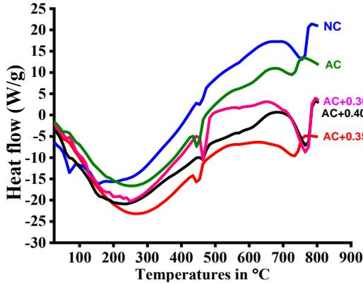
Fig. 8 Differential scanning calorimetry curves of concrete
