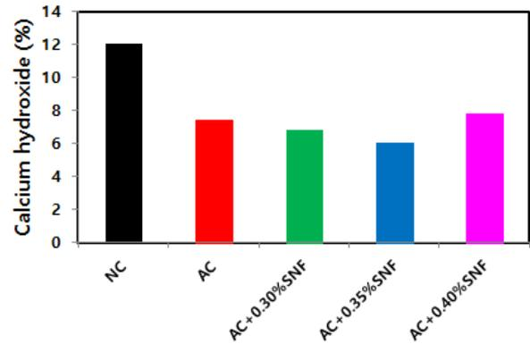
Fig. 12 Calcium hydroxide (%) of various concrete mixes
