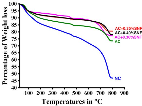
Fig. 9 Percentage of weight loss curves of the concrete
