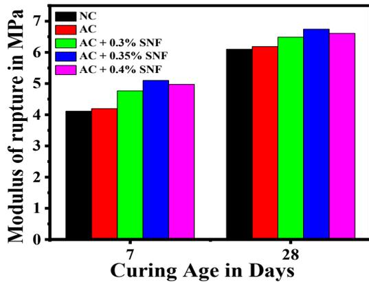
Fig. 5 Modulus of rupture values of concrete mixes
