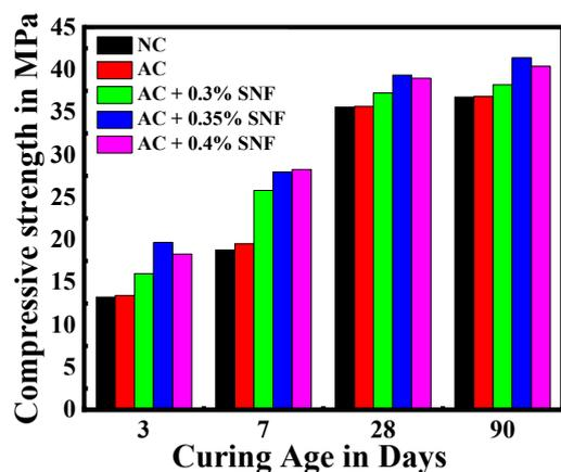
Fig. 3 Compressive strength variation of different mixes with age
