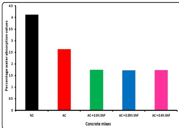
Fig. 6 Water absorption test results different concrete mixes
