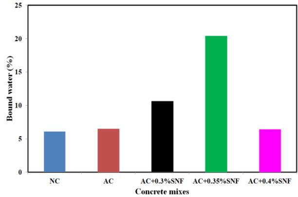
Fig. 11 Bound water (%) of different concrete mixes
