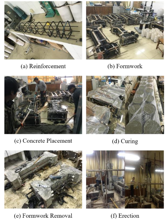
Fig. 2 Production of test specimens
