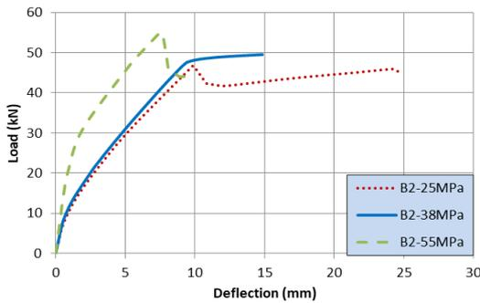
Fig. 20 Effect of compressive strength on the behavior of single spliced smooth bars beams
