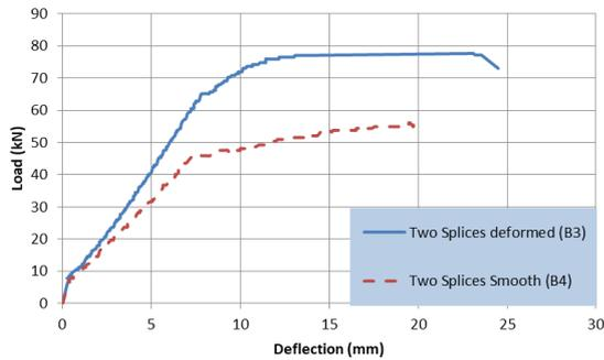
Fig. 8 Load deflection curves for the tested beams reinforced with two spliced bars and single bar non-spliced
