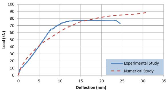
Fig. 15 Load deflection curves for the tested beam B3
