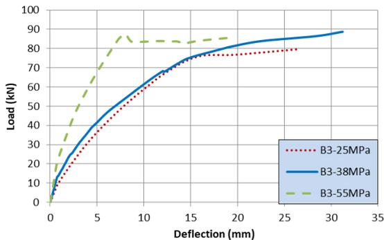
Fig. 21 Effect of compressive strength on the behavior of two spliced deformed bars beams
