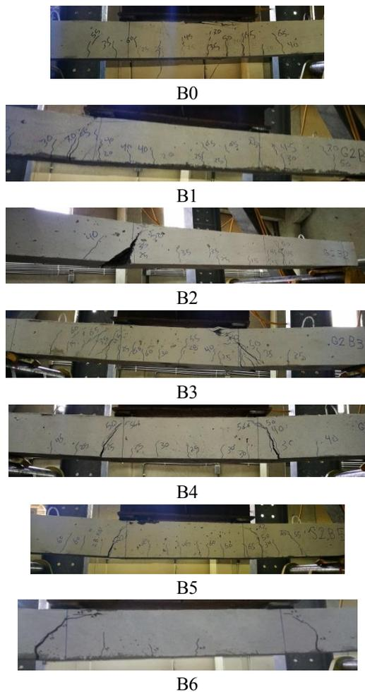
Fig. 4 Crack pattern for the tested beams
