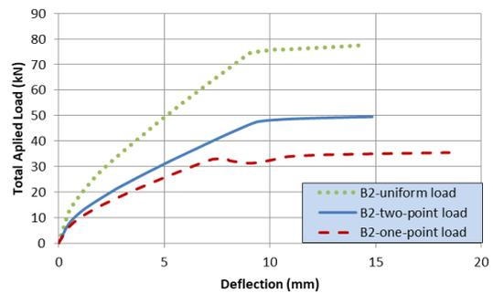
Fig. 24 Effect of load type on the behavior of single spliced smooth bars beams
