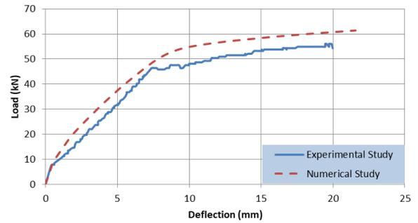
Fig. 16 Load deflection curves for the tested beam B4
