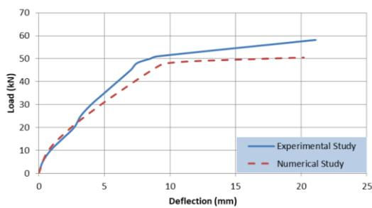
Fig. 14 Load deflection curves for the tested beam B2
