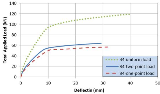
Fig. 26 Effect of load type on the behavior of two spliced smooth bars beams
