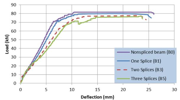
Fig. 5 Load deflection curves for the tested beams reinforced with deformed bars
