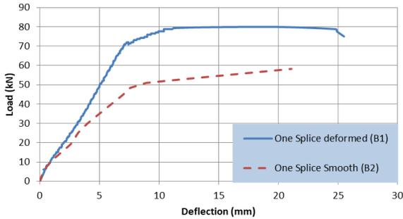
Fig. 7 Load deflection curves for the tested beams reinforced with single spliced bar and the two bars non-spliced
