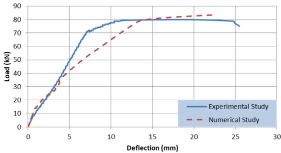
Fig. 13 Load deflection curves for the tested beam B1
