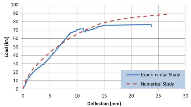
Fig. 17 Load deflection curves for the tested beam B5
