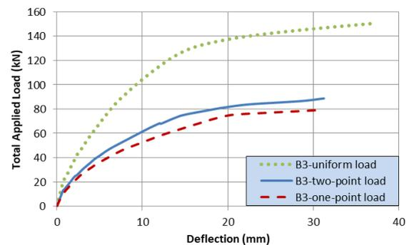
Fig. 25 Effect of load type on the behavior of two spliced deformed bars beams
