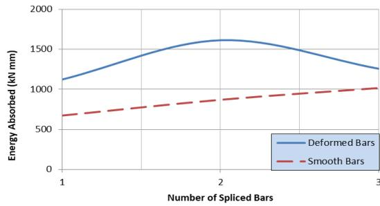
Fig. 12 Effect of number of spliced bars on energy absorbed
