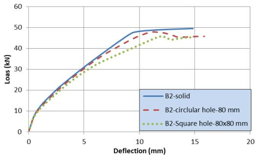
Fig. 28 Effect of hole shape on the behavior of single spliced smooth bars beams
