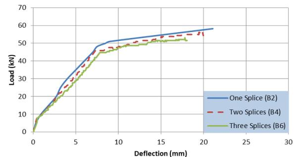
Fig. 6 Load deflection curves for the tested beams reinforced with smooth bars
