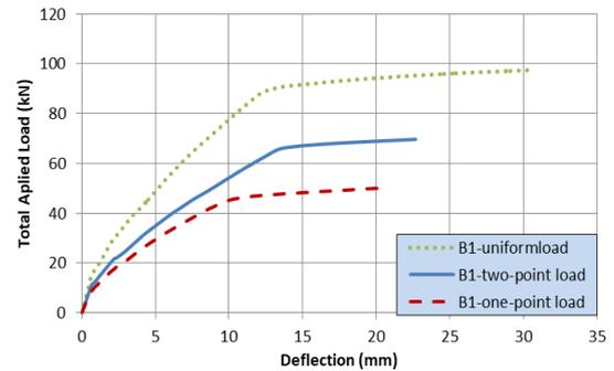
Fig. 23 Effect of load type on the behavior of single spliced deformed bars beams
