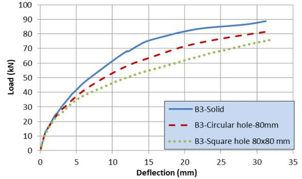
Fig. 29 Effect of hole shape on the behavior of two spliced deformed bars beams
