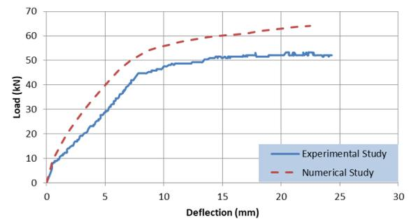
Fig. 18 Load deflection curves for the tested beam B6
