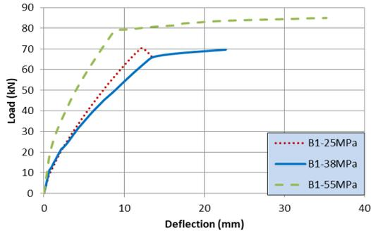
Fig. 19 Effect of compressive strength on the behavior of single spliced deformed bars beams
