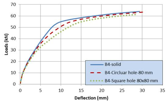
Fig. 30 Effect of hole shape on the behavior of two spliced smooth bars beams
