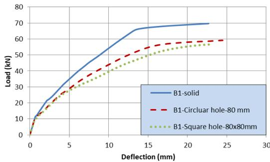
Fig. 27 Effect of hole shape on the behavior of single spliced deformed bars beams
