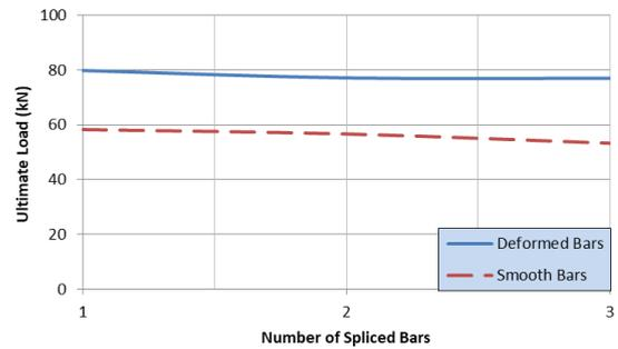
Fig. 10 Effect of number of spliced bars on ultimate loads
