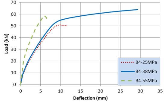
Fig. 22 Effect of compressive strength on the behavior of two spliced smooth bars beams
