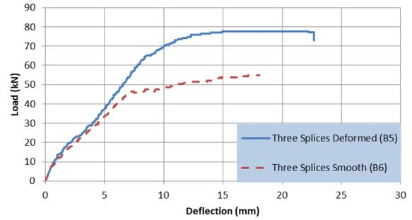
Fig. 9 Load deflection curves for the tested beams reinforced with three spliced bars
