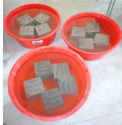
Fig. 2 Concrete cubes prepared by using different mixing approaches immersed in 1% of sulphuric acid solution for curing
