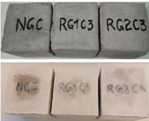
Fig. 23 State of concrete specimens after 270 days of immersion in MgSO_4 (5%) solution
