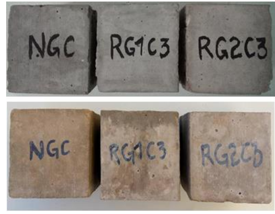
Fig. 24 State of concrete specimens after 270 days of immersion in NaCl (5%) solution
