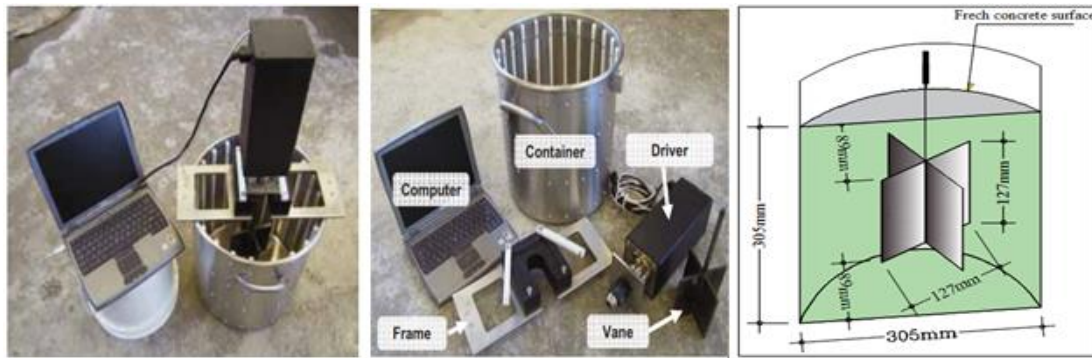
Fig. 5 Principal parts of the rheometer test (ICAR type Rheometer)
