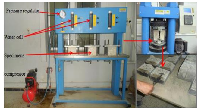
Fig. 6 Measurements of the depth of water penetration inside the different types of concrete
