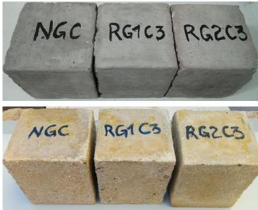
Fig. 22 State of concrete specimens after 270 days of immersion in H_2SO_4 (5%) solution
