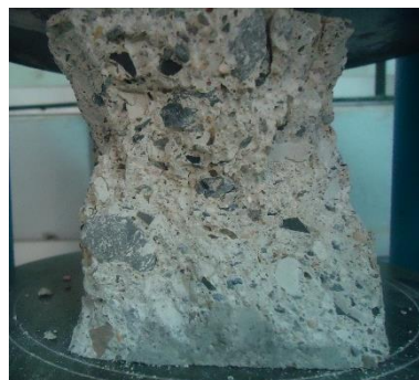
Fig. 2 Typical compression failure of concrete cylinder, showing non-crushed aggregate particles
