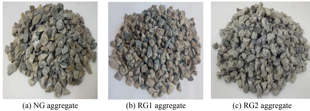
Fig. 3 Typical natural and recycled concrete aggregates
