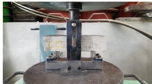
Fig. 6 Flexural strength test set-up
