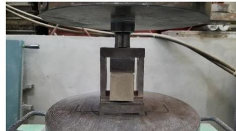
Fig. 5 Compressive strength test set-up
