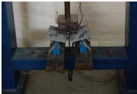
Fig. 4 Flexural specimen after failure
