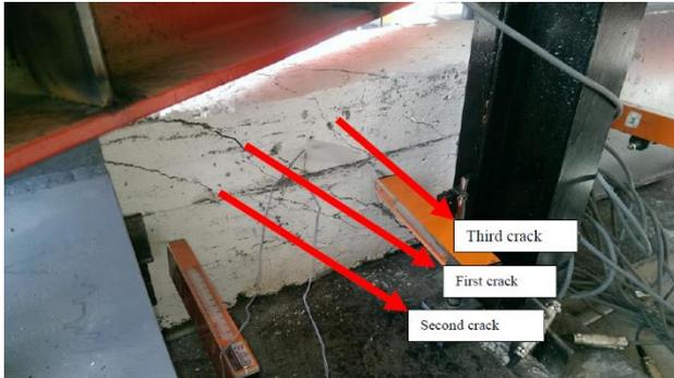
Fig. 4 The first second and third cracks in the tested beam
