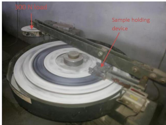
Fig. 2 Experimental setup for measurement of abrasion resistance of concrete
