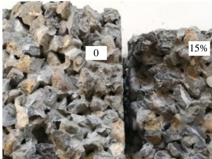
Fig. 4 The cross section of PCPC specimen with 0 and 15% fine aggregate
