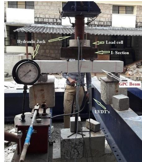
Fig. 1 Detailed test setup of RGPC beam under two-point loading
