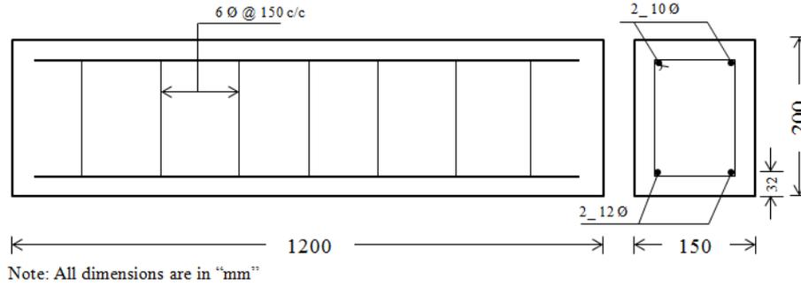
Fig. 2 Geometry and cross section of tested beam
