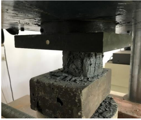
Fig. 9 Compressive strength testing of 28 days cured UHP-HFRC- 2 sample (Phase- III)
