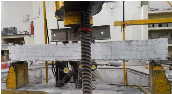
Fig. 9 Typical view of static load test setup
