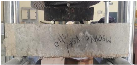
Fig. 8 Failure pattern of prismatic beam
