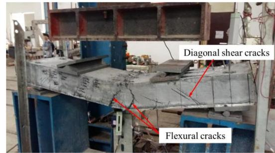
Fig. 5 Typical failure mode of test specimen S2-A-1
