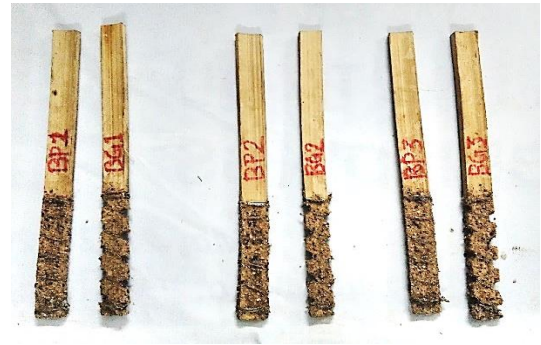
Fig. 4 Bond-Tite coating with sand particles
