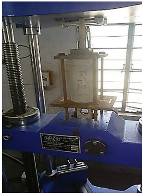
Fig. 11 Pull-out sample placed inside UTM
