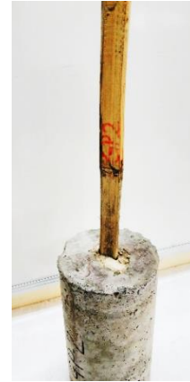
Fig. 13 Bond failure of untreated plain bamboo
