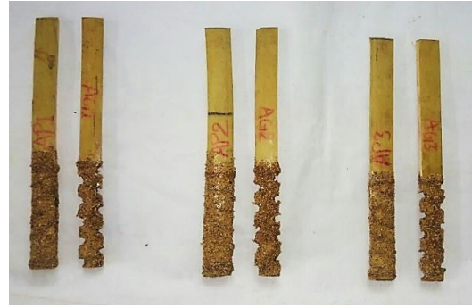
Fig. 3 Triflor PUAL lacquer coating with sand particles
