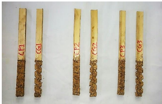
Fig. 5 Araldite coating with sand particles
