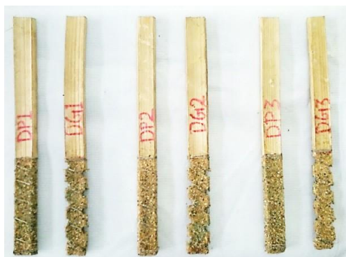
Fig. 6 Epoxy coating with sand particles
