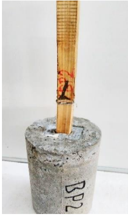
Fig. 16 Bond failure of treated plain bamboo
