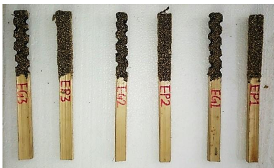
Fig. 7 Bitumen (VG-30) coating with sand particles
