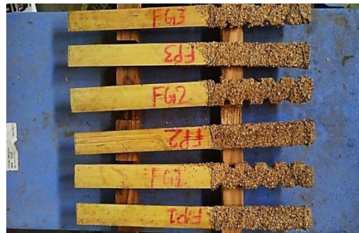
Fig. 8 EPI BOND -21 coating with sand particles
