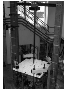
(c) Drop-weight test device (Hrynyk and Vecchio 2014)
