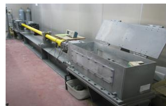
(a) Nitrogen gas gun test device, Chungnam National University (Lee et al. 2018)
