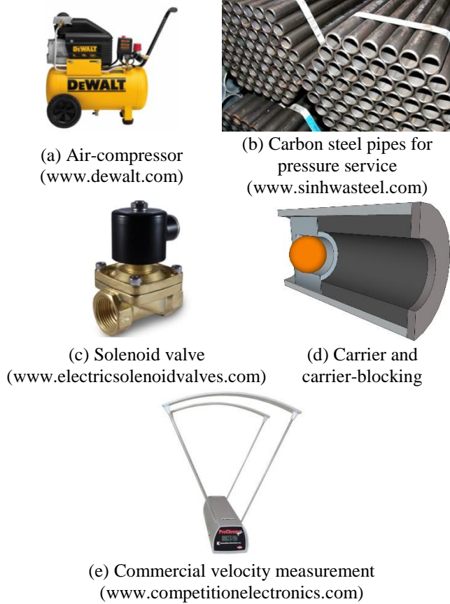
Fig. 2 Key equipment for small impact test device development
