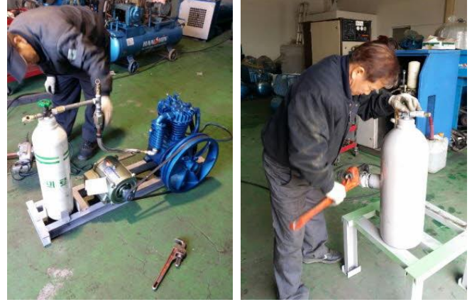
Fig. 5 Manufacturing air compressor and air tank system
