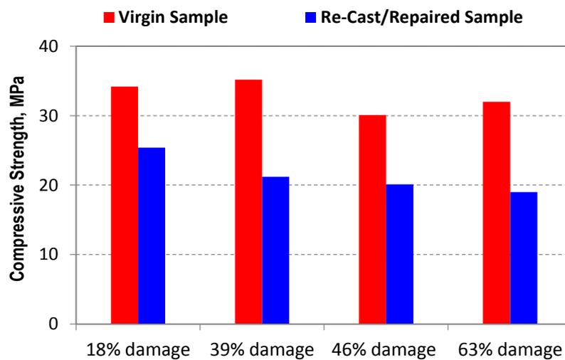
Fig. 10 Compressive strength of control and re-cast samples
