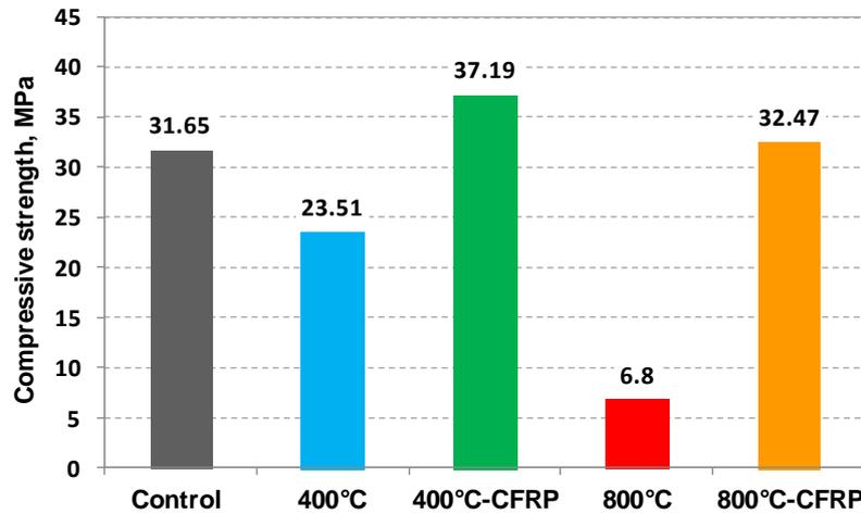
Fig. 13 Compression strength: effect of elevated temperature and strengthening
