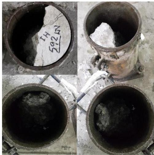
Fig. 5 Intact concrete placed in mold for re-concreting
