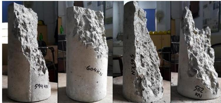
Fig. 1 Intact pieces of specimens fully damaged in compression
