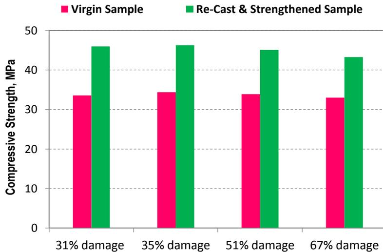
Fig. 12 Compressive strength of control and strengthened re-cast samples
