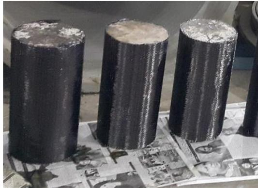
Fig. 7 Concrete cylinder strengthened using CFRP sheets
