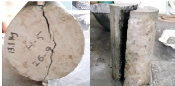
Fig. 2 Cylinder subjected to split tensile loading
