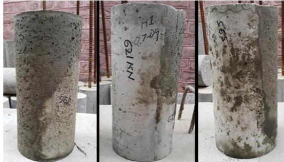
Fig. 6 Re-cast concrete cylinders
