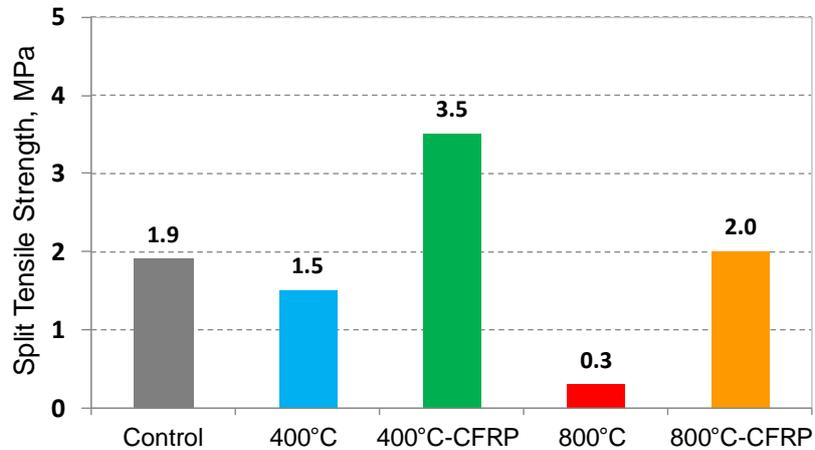
Fig. 18 Split tensile strength: effect of elevated temperature and strengthening
