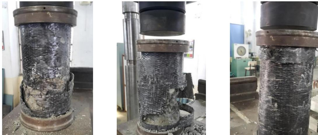
Fig. 15 Failure mode in compression (re-cast & strengthened specimens)
