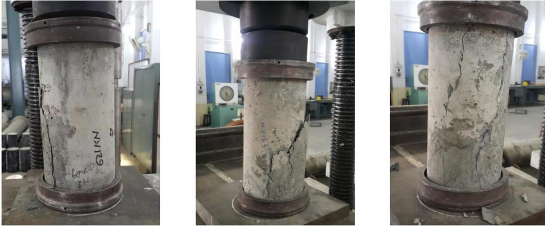
Fig. 14 Failure mode in compression (re-cast samples)
