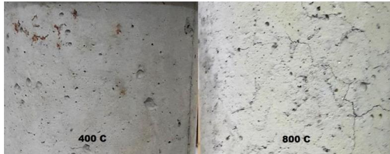
Fig. 4 Surface condition of samples after exposure to elevated temperature
