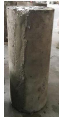
Fig. 9 Specimen after joining with mortar
