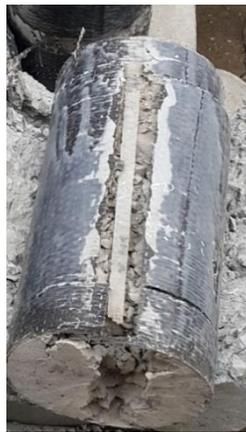
Fig. 19 Failure mode in splitting tensile test
