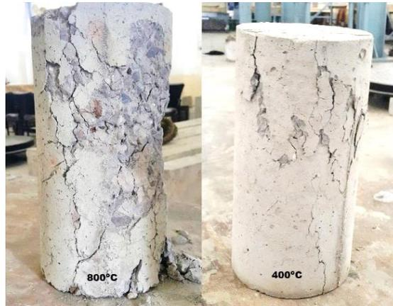
Fig. 16 Failure mode in compression (heated samples)
