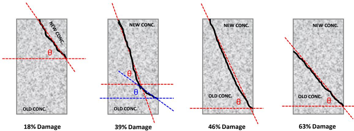
Fig. 11 Angle of failure surface with horizontal
