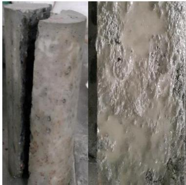
Fig. 8 Cement slurry applied on the inner surfaces of concrete cylinder
