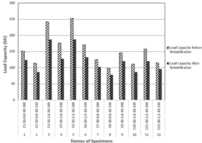
Fig. 7 Ultimate load capacity of all corbels before and after the rehabilitation by BFM
