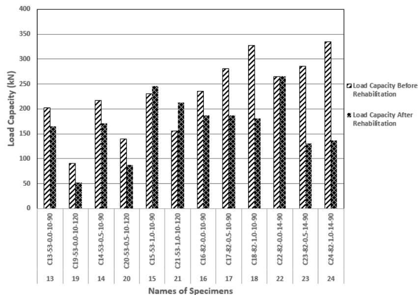
Fig. 11 The behaviour of part two of second group after rehabilitation by BFM with respect to the ultimate load capacity
