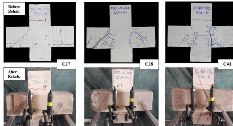
Fig. 12 Mode of failure for several corbels before and after the rehabilitation.
