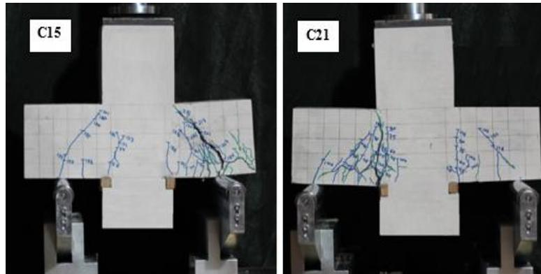
Fig. 9 Mode of failure of C15 was Diagonal splitting failure and C21 was flexural failure
