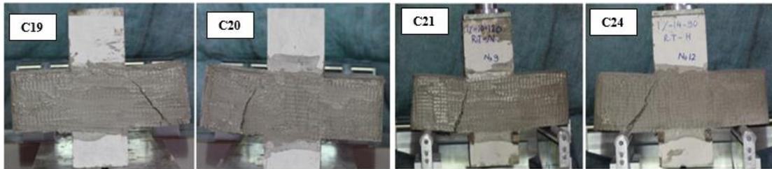
Fig. 10 Failure mode of Basalt Fiber Mesh in several corbels of part two of second group (Ruptured in BFM)
