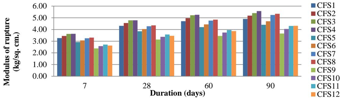
Fig. 9 Flexural strength of flyash admixed ternary concrete mixes
