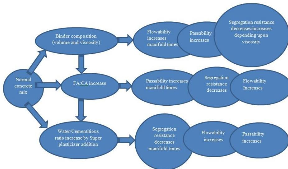
Fig. 2 Sequential steps in yielding a SCC from a normal concrete
