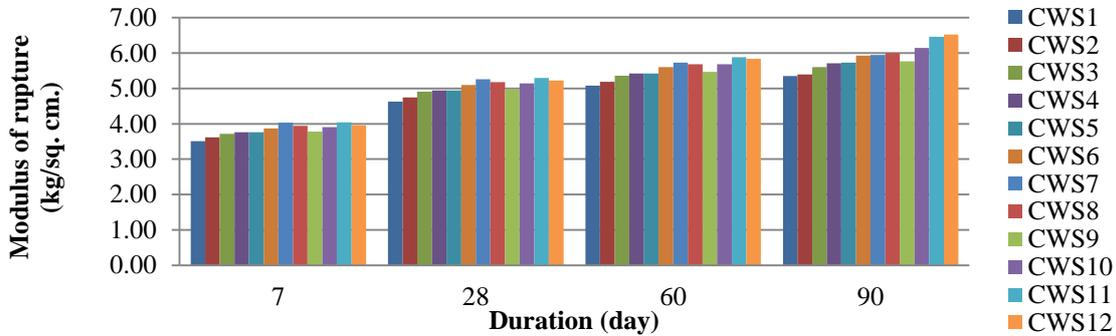
Fig. 10 Flexural strength of WMF admixed ternary concrete mixes
