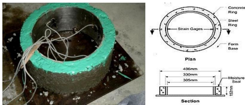
Fig. 3 Configuration of restrained SCC ring samples
