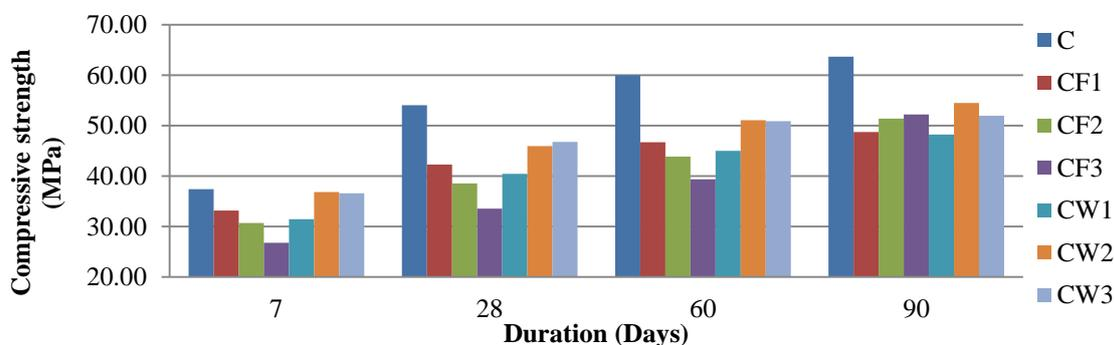
Fig. 5 Compressive strength of normal and binary concrete mixes
