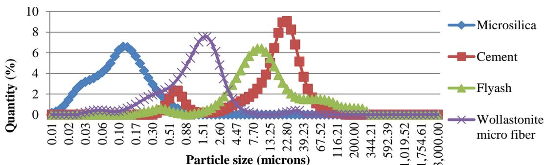
Fig. 1 Particle size distribution of WMF, flyash cement and microsilica
