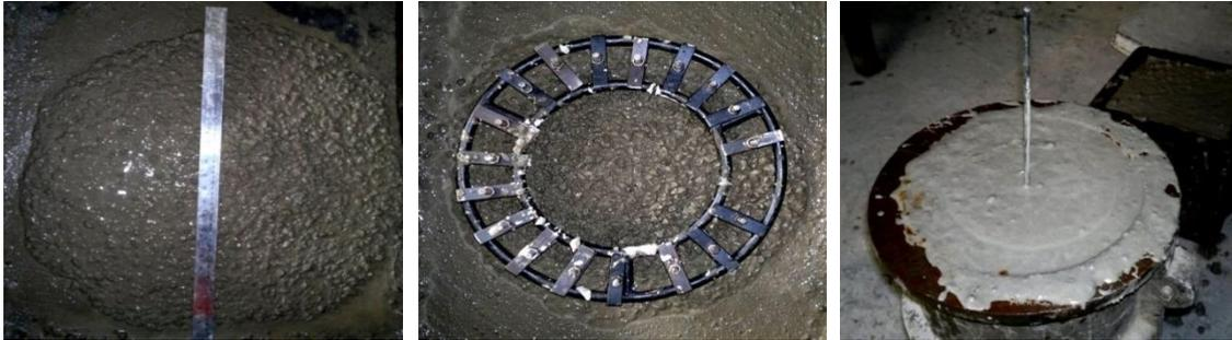
Fig. 3 Workability test for (a) flowability, (b) passability and (c) segregation resistance
