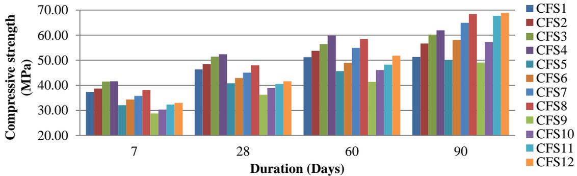
Fig. 6 Compressive strength of flyash admixed ternary concrete mixes
