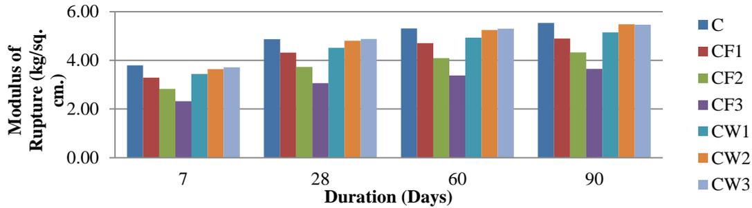
Fig. 8 Flexural strength of normal concrete mix and binary concrete mixes
