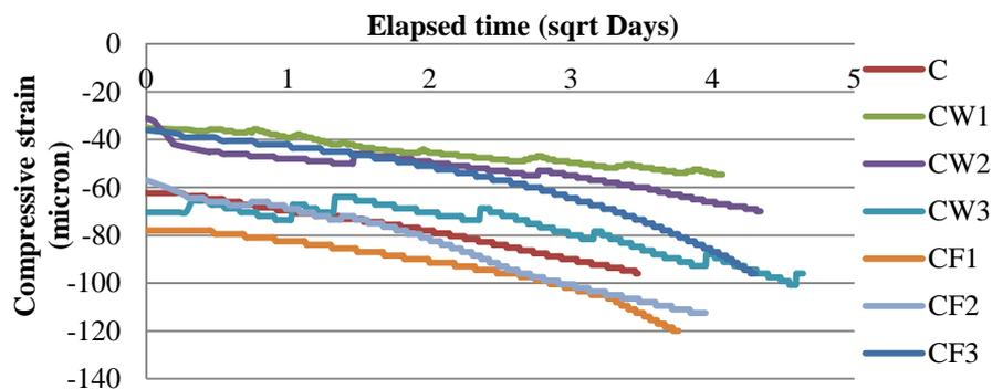
Fig. 4 Compressive strain data with respect to square root of elapsed time for concrete mixes
