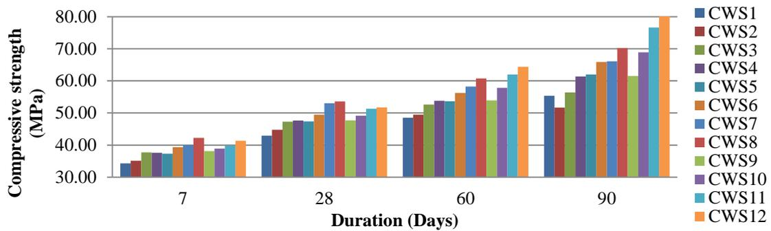
Fig. 7 Compressive strength of WMF admixed ternary concrete mixes
