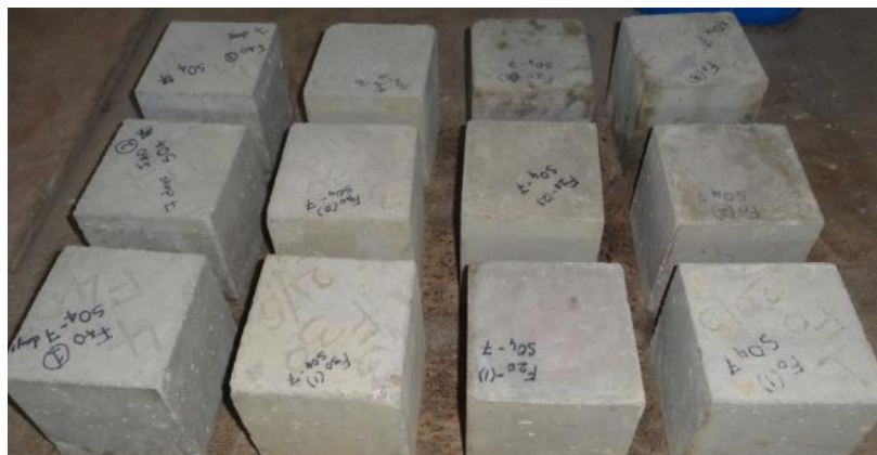
Fig. 2 Concrete cubes after sulphate attack
