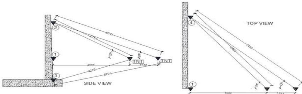
Fig. 18 Detailed plots of gauges on façade of the wall and TNT
