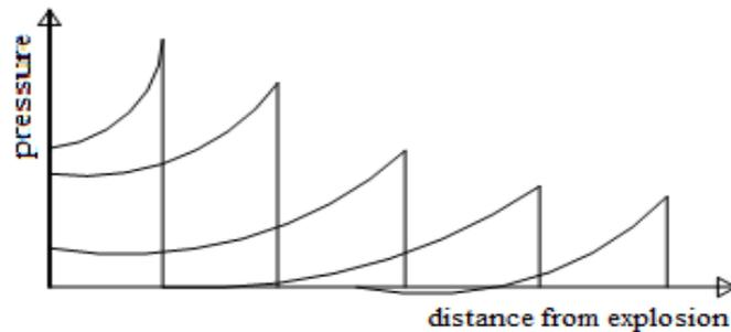
Fig. 2 Pressure wave-distance interaction related to blasting
