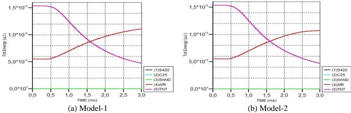
Fig. 22 Total energy values of the models after explosion
