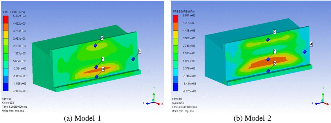
Fig. 20 Pressure contour diagram of the models
