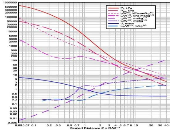
Fig. 4 Parameters of positive phase of shock spherical wave of TNT charges from free-air bursts
