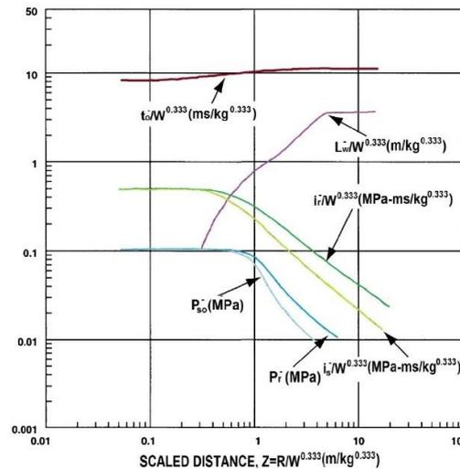
Fig. 9 Parameters of negative phase of shock wave of TNT charges
