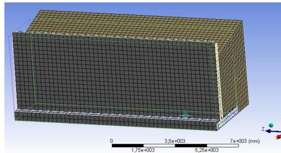
Fig. 16 3D Geometrical model of the RC retaining wall designed in ANSYS Workbench
