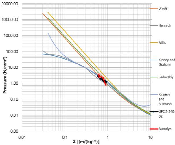
Fig. 23 Pressure values of different equations, proposes and autodyn for general Z values
