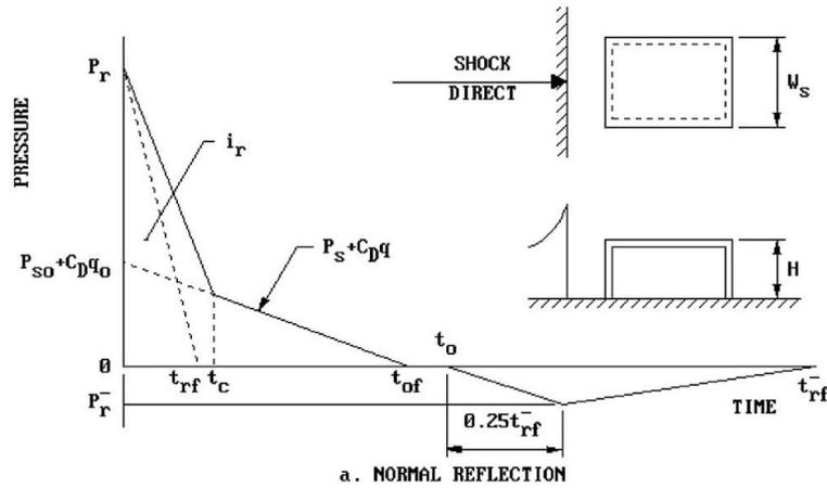
Fig. 6 Triangular assumption form of pressure time history graph
