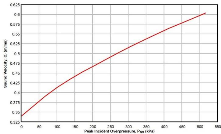
Fig. 7 Sound velocity in reflected overpressure graph
