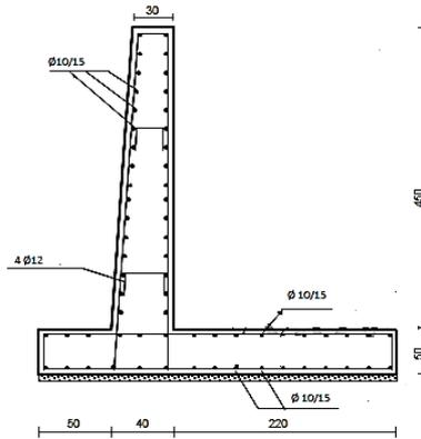
Fig. 15 3D Geometrical dimensions of the RC retaining wall (dimensions, cm)
