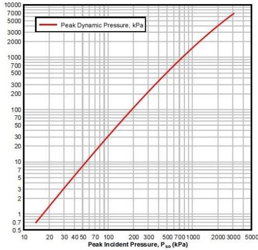
Fig. 8 Peak dynamic pressure-peak incident pressure graph
