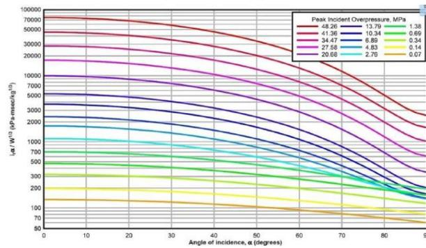
Fig. 12 Calculation of scaled reflected impulse due to angle
