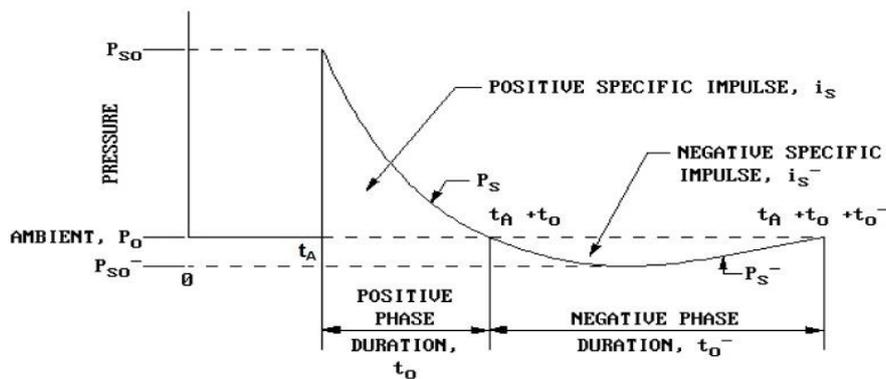
Fig. 3 Pressure wave-distance interaction related to blasting
