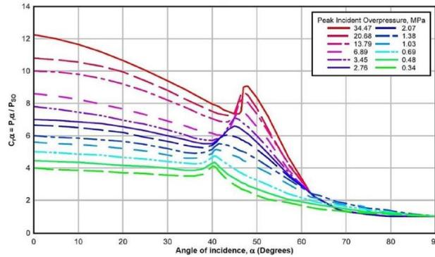
Fig. 11 Calculation of scaled reflected pressure coefficient due to angle
