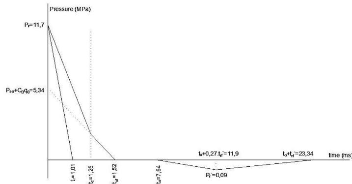
Fig. 24 Idealized equivalent triangular pressure-time graph
