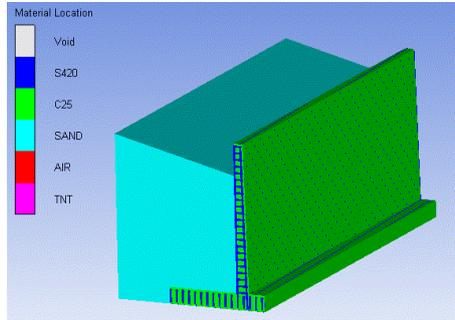
Fig. 14 3D Drawing model of the RC Retaining wall
