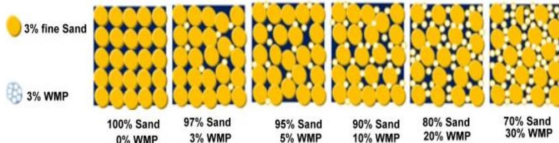
Fig. 2 Graphical distribution of different contents of WMP in 1 mm<sup>2</sup> of PC
