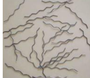
Fig. 2 Crimped steel fibers
