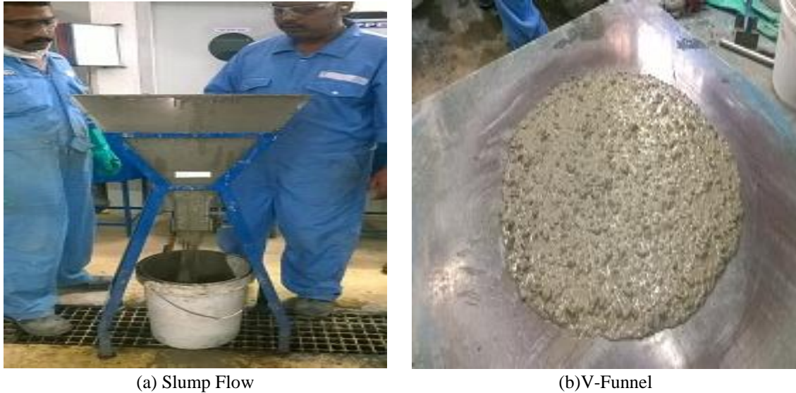
Fig. 3 V-funnel, flow table, ICAR Rheometer used for the testing
