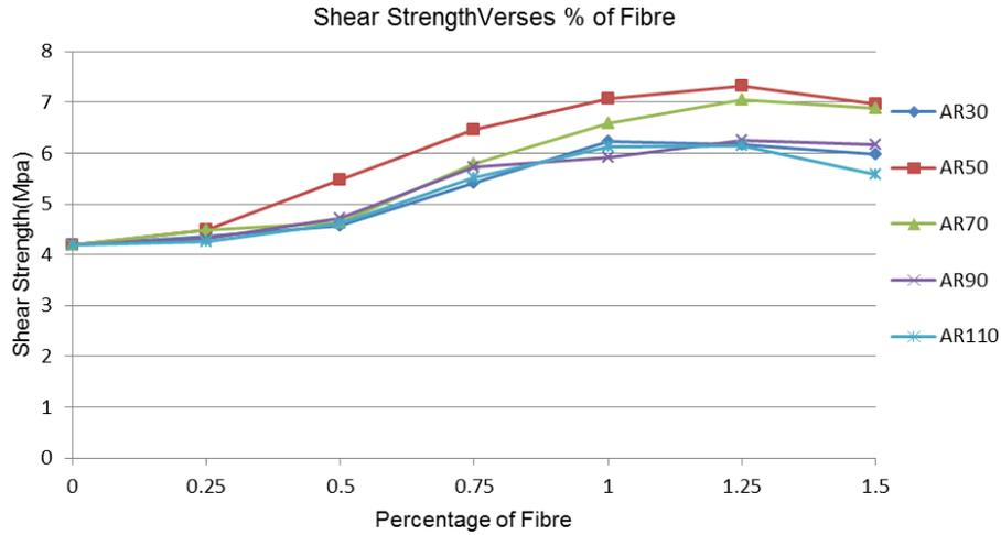
Fig. 7 Shear strength variation with percentage of fibre
