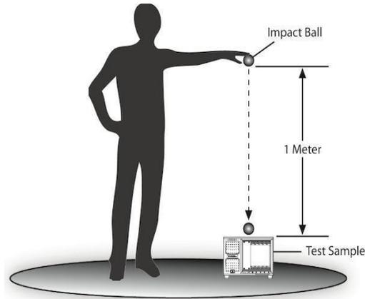
Fig. 4 Impact test
