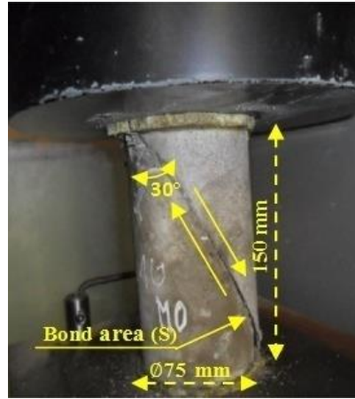
Fig. 3 slant-shear specimen under compression testing
