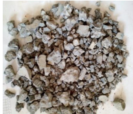
(b) Broken concrete fragments
