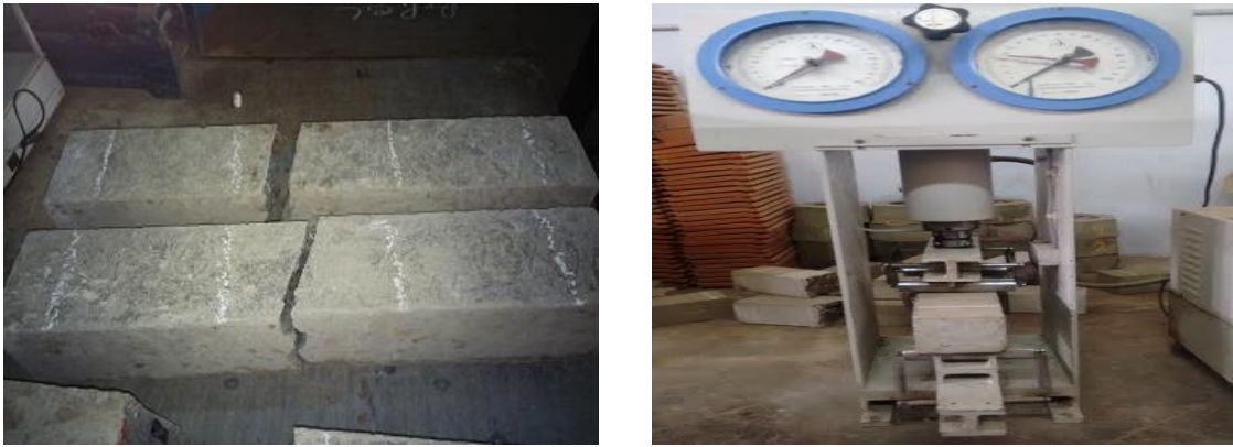
Fig. 13 Flexural Strength arrangement and cracked beams
