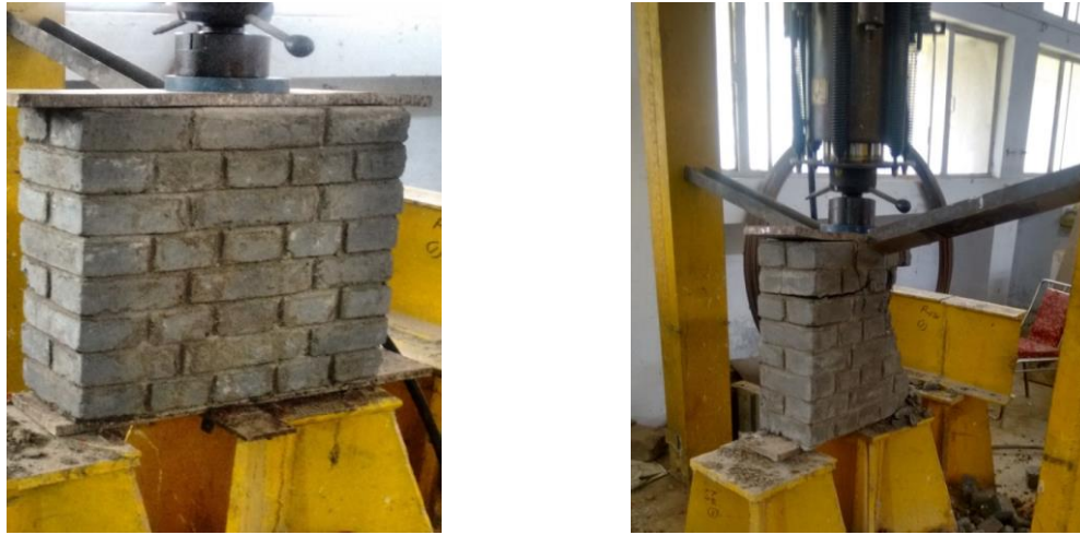
(a) Brick prism of coal ash bricks before loading
