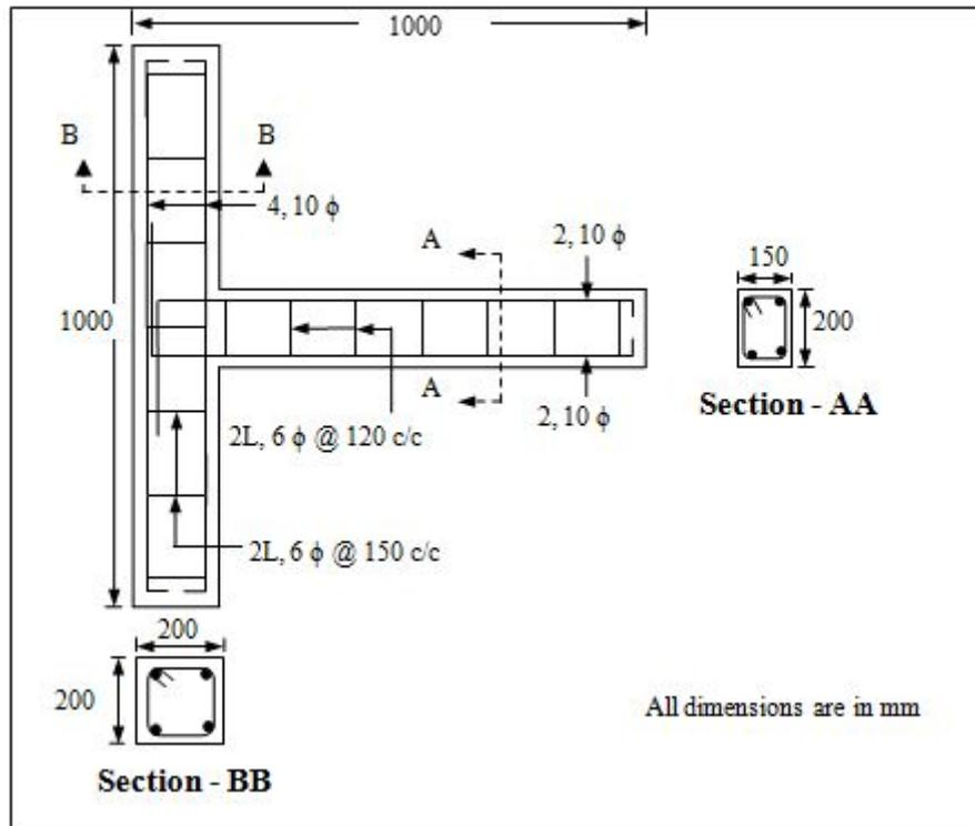
Fig. 1 Dimension and reinforcement details of specimens
