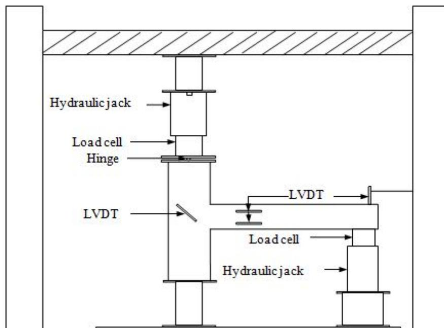
Fig. 2 Schematic diagram of test setup
