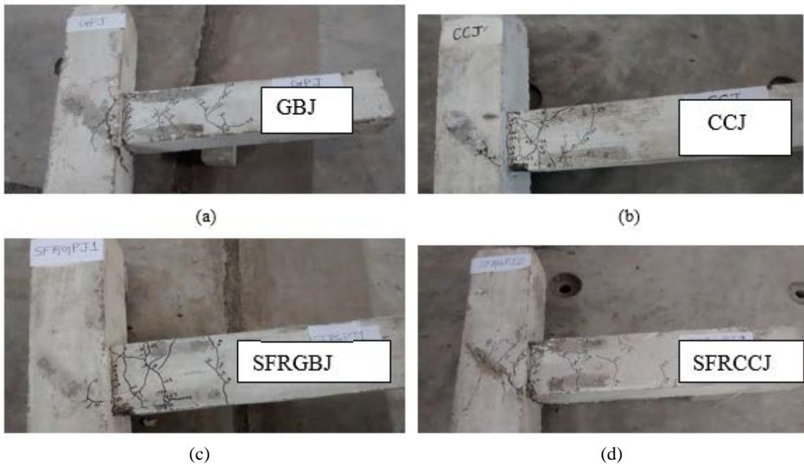
Fig. 4 Crack pattern of specimens
