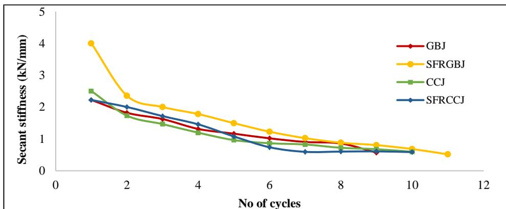
Fig. 8 Stiffness degradation
