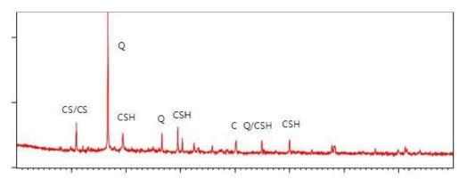
Fig. 8 X-Ray Diffraction of MX1 at the curing ages of 28 days (Q = quartz; CS = calcium silicate; C = calcite; CSH = calcium silicate hydrate)
