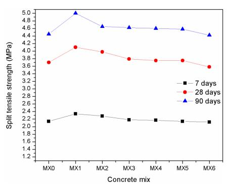
Fig. 2 Split tensile strength of concrete at the curing ages of 7, 28 & 90 days
