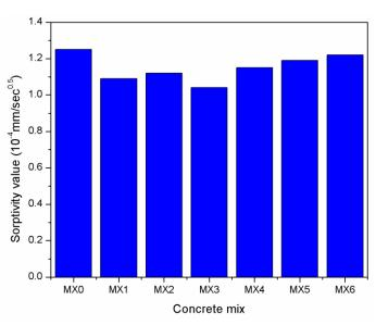
Fig. 6 Sorptivity of concrete at the curing ages of 28 days
