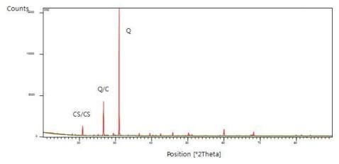
Fig. 7 X-Ray Diffraction of MX0 at the curing ages of 28 days (Q = quartz; CS = calcium silicate; CSH = calcium silicate hydrate)
