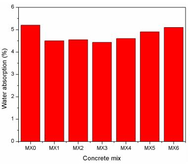
Fig. 5 Water absorption of concrete at the curing ages of 28 days
