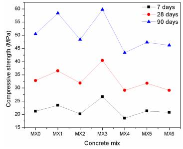
Fig. 1 Compressive strength of concrete at the curing ages of 7, 28 & 90 days
