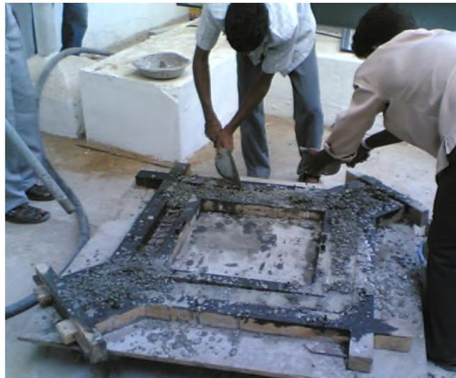
Fig. 2 Specimens concreting and vibrating
