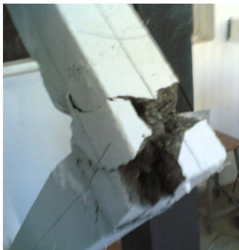
Fig. 8 Typical plastic hinge pattern
