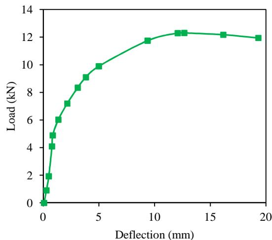
Fig. 4 Load-displacement profile of BFC1 specimens
