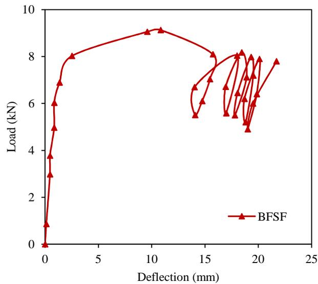
Fig. 9 Load - displacement profile of BFSF specimens
