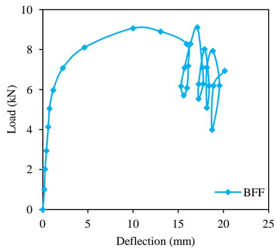
Fig. 7 Load – displacement profile of BFF specimens
