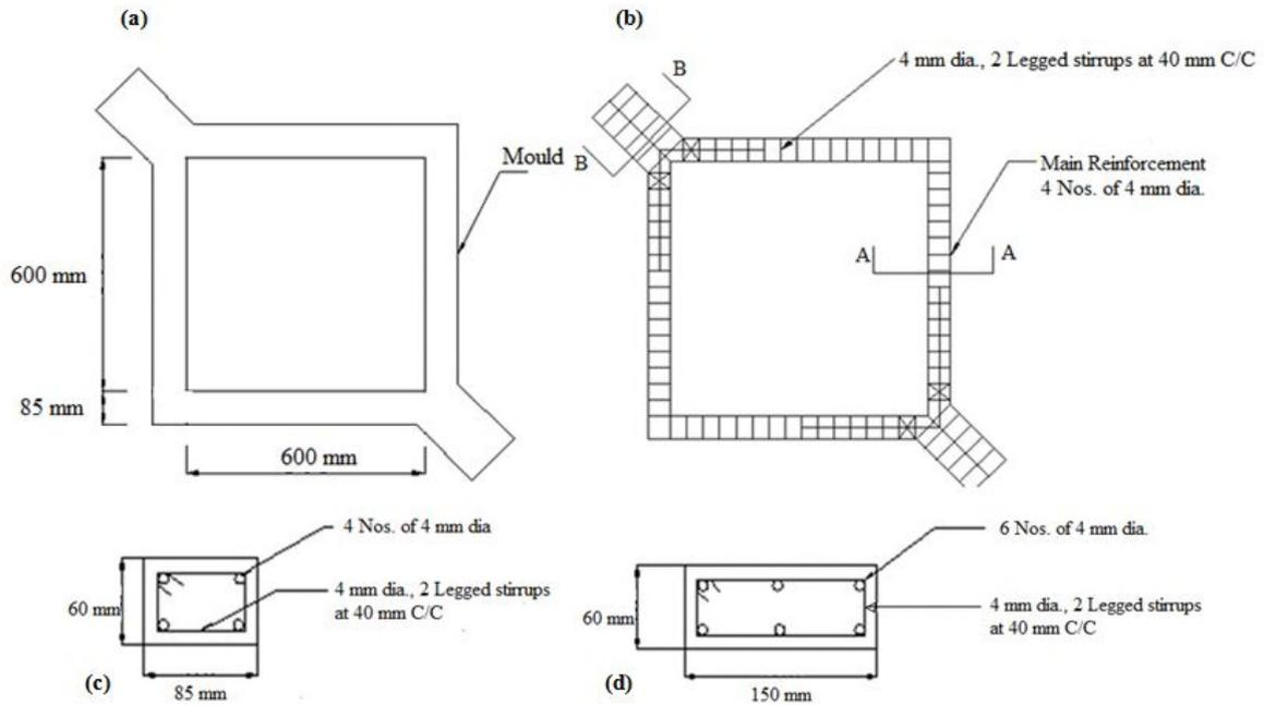
Fig. 1 Schematics of (a) mould (b) reinforcement (c) cross section AA and (d) cross section BB
