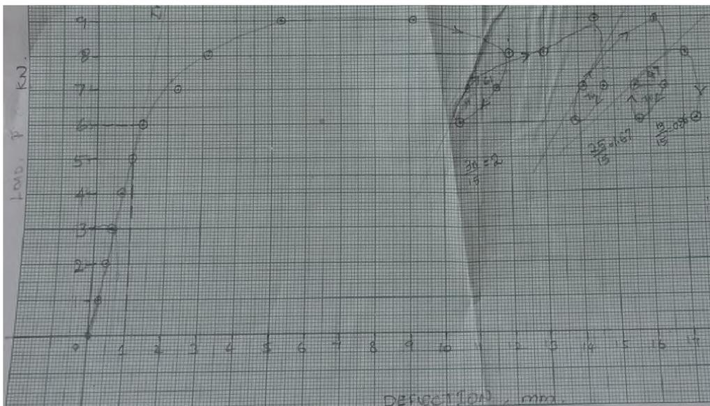
Fig. 6 Plot showing Initial stiffness, slope and ultimate load of BFC2 specimens
