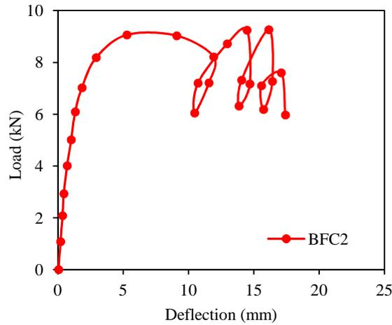
Fig. 5 Load-displacement profile of BFC2 specimens
