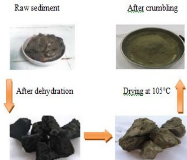
Fig. 4 Sediment preparation for geotechnical characterization
