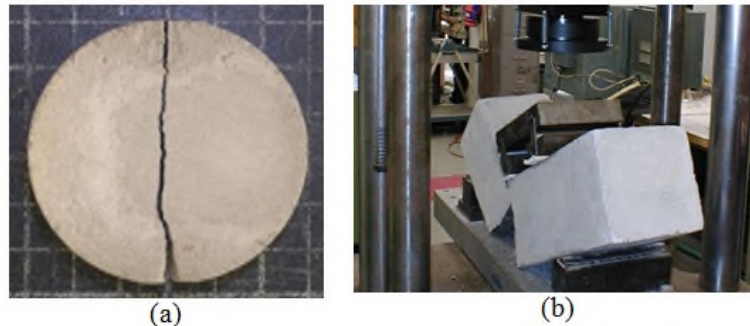
Fig. 8 tensile failure of specimens in, a) Splitting test and b) three point load test
