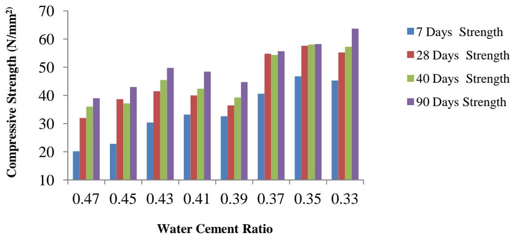
Fig. 2 Variation in compressive strength with water cement ratio
