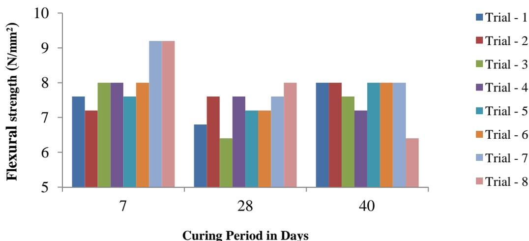
Fig. 4 Variation in flexural strength with curing period
