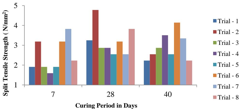
Fig. 5 Variation in split tensile strength with curing period
