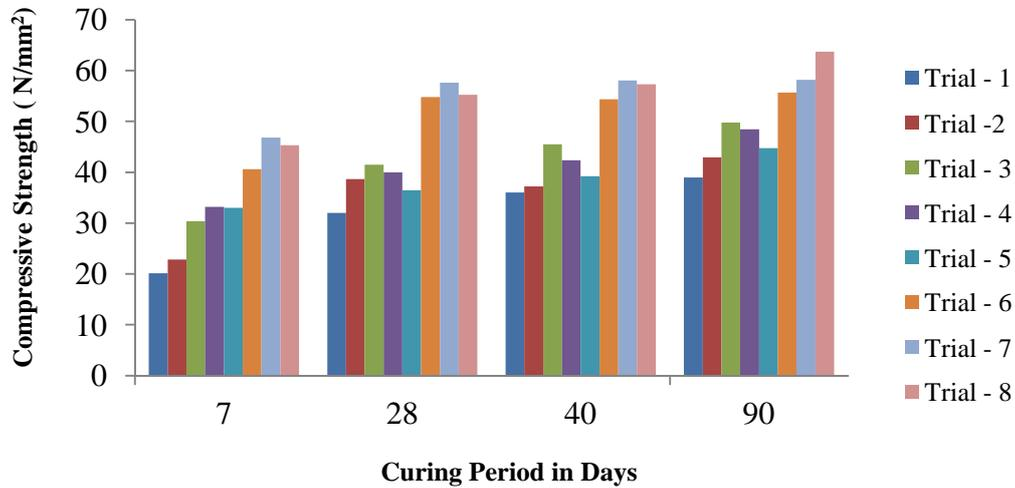
Fig. 1 Variation in compressive strength with curing period for different trial mixes
