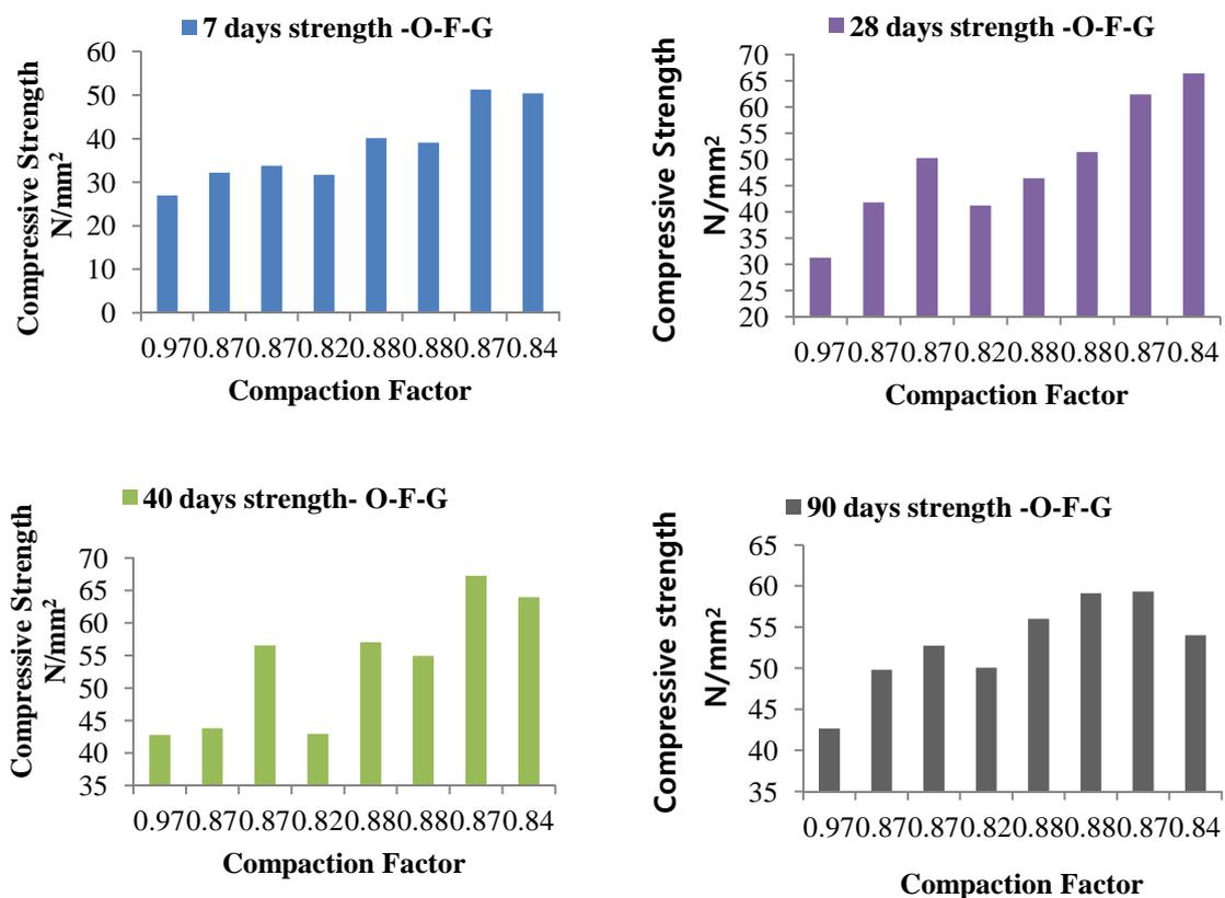
Fig. 3: Variation in compressive strength with compaction factor (7, 28, 40 and 90 days' curing period)
