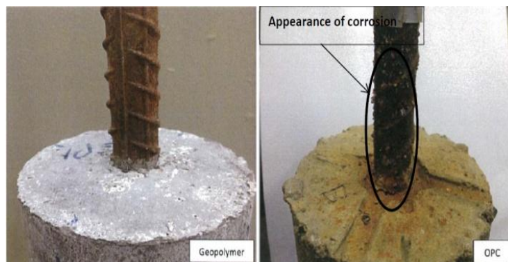
Fig. 6 Corrosion of steel bar in geopolymer concrete and ordinary concrete
