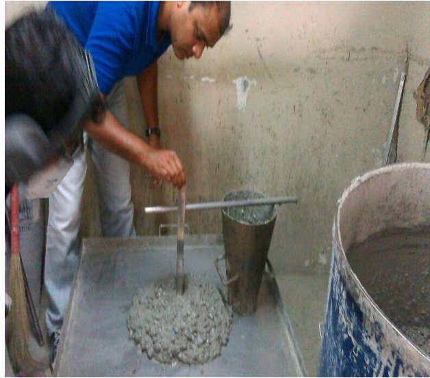
Fig. 1 Slump measurement of fresh concrete
