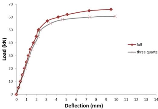
Fig. 7 Load-Deflection behavior without and with FCJ at 75% height
