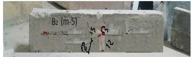
Fig. 11 Failure mode of beam with FCJ at the 0.50 height (B2-M-5)
