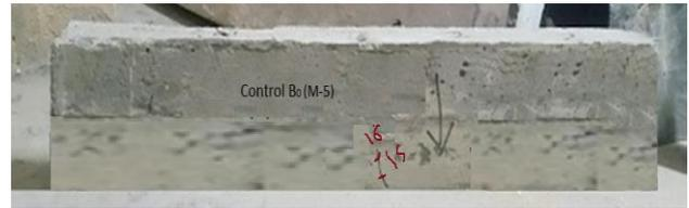
Fig. 9 Failure mode of beam without FCJ (B0-M-5)
