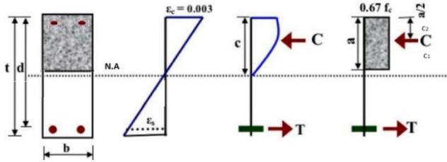
Fig. 13 Stress and strain diagram
