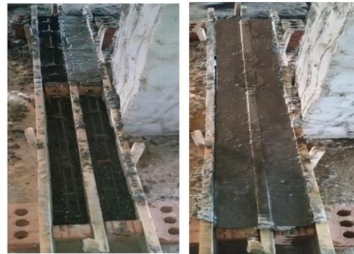
Fig. 3 Step casting with FCJ 25, 50, 75 and 100 of samples height
