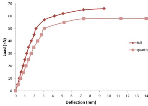
Fig. 5 Load-deflection behavior without and with FCJ at 25% height
