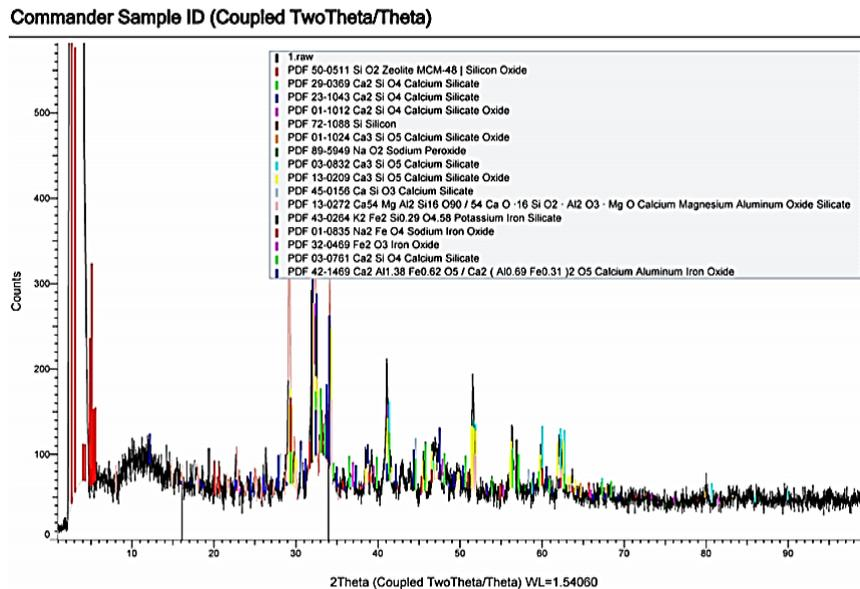
Fig. 2 XRD image of CW (Heniegal *et al.* 2017)
