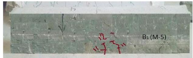
Fig. 10 Failure mode of beam with FCJ at the 0.25 height (B1-M-5)
