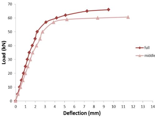
Fig. 6 Load-deflection behavior without and with FCJ at 50% height
