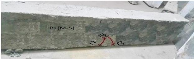
Fig. 12 Failure mode of beam with FCJ at the 0.75 height (B3-M-5)
