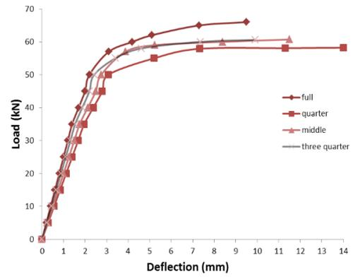
Fig. 8 Comparing load-deflection behavior without and with FCJ at different casting
