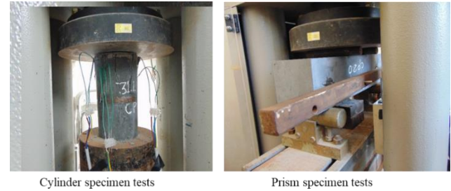
Fig. 3 Specimen tests for obtaining UHPC properties
