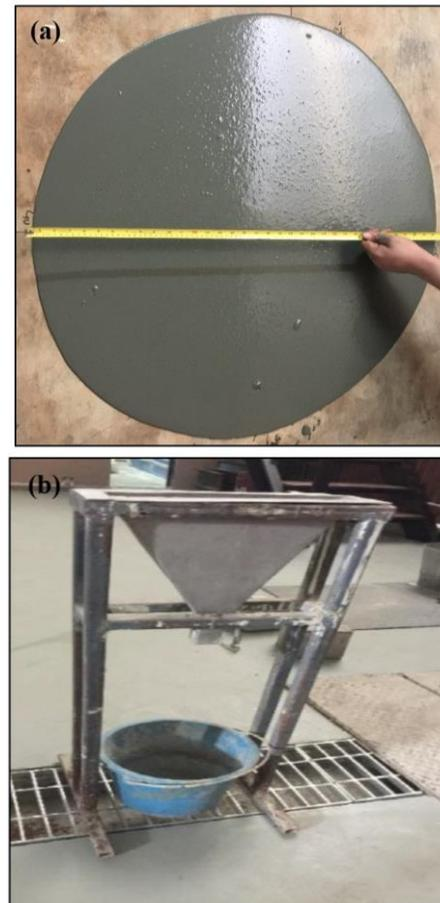
Fig. 3 Measurement of workability of concrete: (a) Slump flow and (b) V-funnel viscosity
