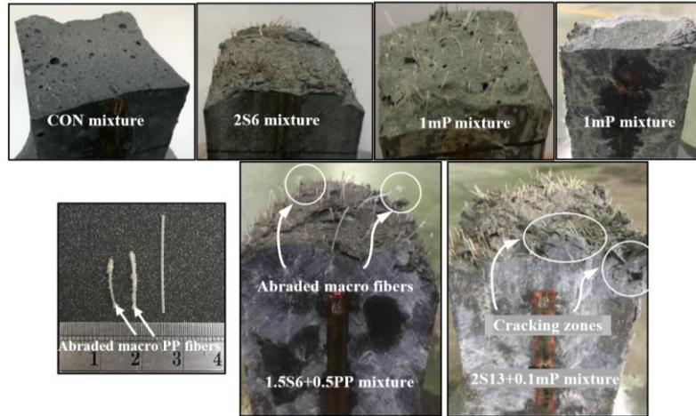
Fig. 11 Sample failure under uniaxial tension
