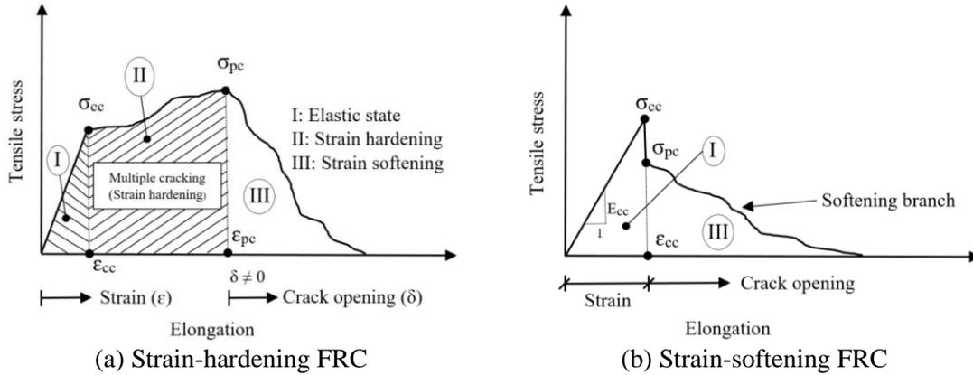
Fig. 1 Tensile behaviour of strain-hardening and strain-softening FRC (Naaman and Reinhardt 2006, Park *et al.* 2012, Wille *et al.* 2014)
