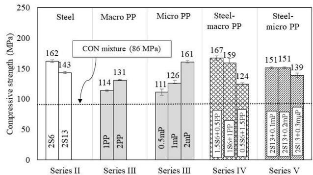
Fig. 6 Compressive strengths of composites made with different types of fibres
