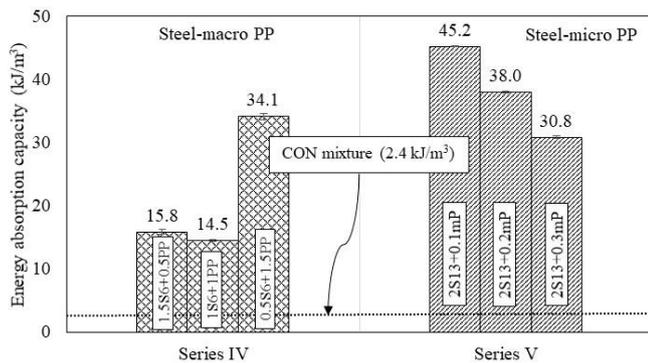
Fig. 9 Energy absorption capacity of hybrid FRCs
