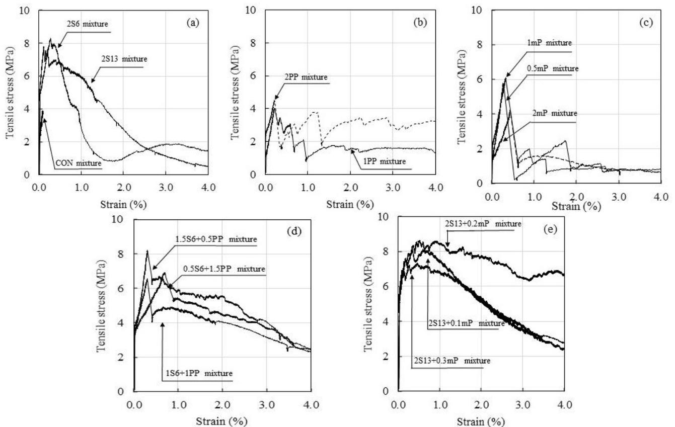
Fig. 7 Mean stress-strain curves obtained from direct tension tests for: (a) Series I and II; (b) Series III (FRC with PP fibres); (c) Series III (FRC with mP fibres); (d) Series IV; and (e) Series V
