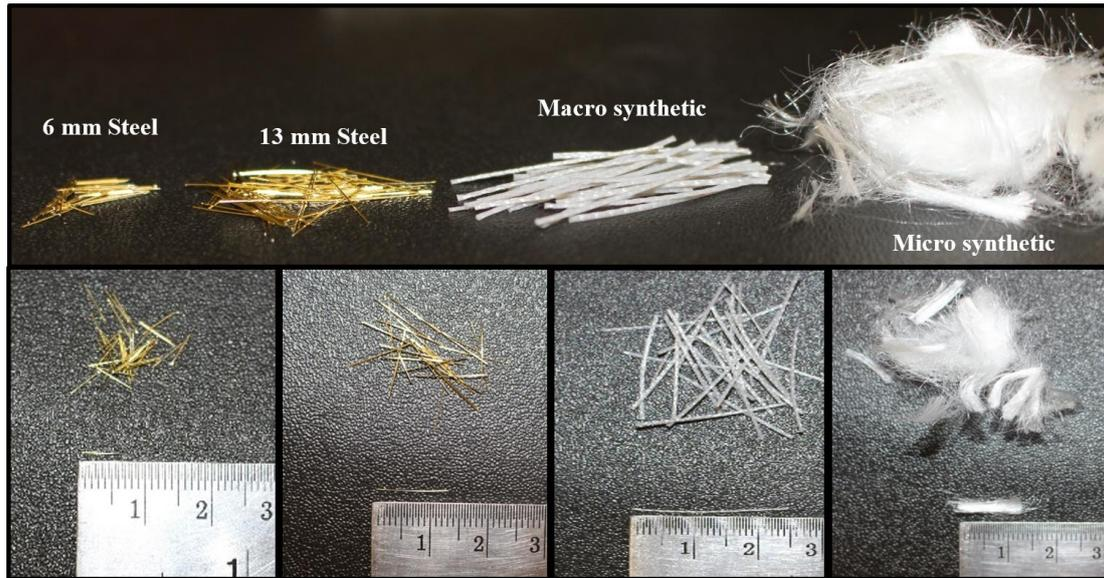
Fig. 2 Steel and synthetic fibres used for FRC preparation
