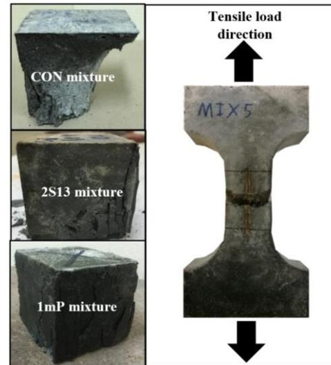
Fig. 10 Failure modes in concrete under stress
