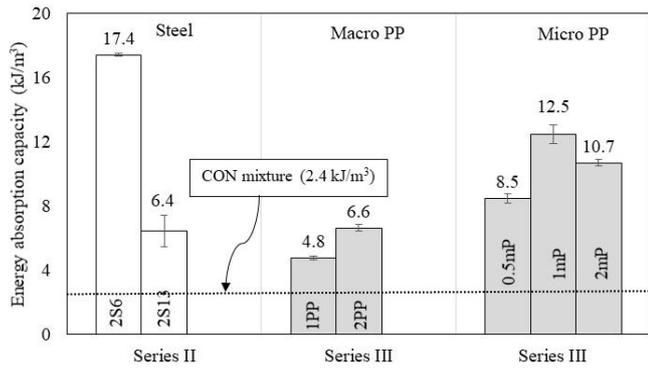
Fig. 8 Energy absorption capacity of single FRCs
