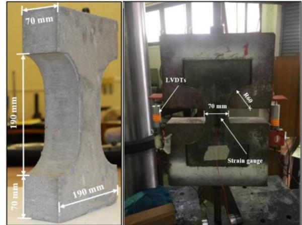
Fig. 5 A dogbone-shaped specimen and experimental set-up
