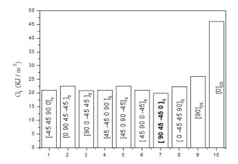
Fig. 5 Effect of plies orientation of the unrepaired plate on the GI values
