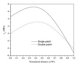
Fig. 15 Distribution of the shear stress tyz along virtual line in adhesive layer
