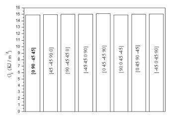
Fig. 7 Effect of plies orientation of the patch on the GI values
