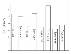
Fig. 18 Effect of plies orientation of the repaired plate on the GI+GII values ( $\theta = 45^{\circ}$ , 2a = 50 mm)
