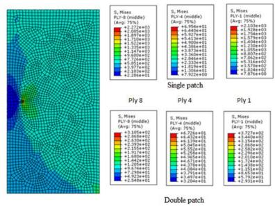
Fig. 10 Contour of Von Mises stresses (MPa) in the various layers of the plate
