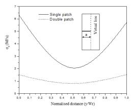
Fig. 14 Distribution of the peeling stress  $\sigma z$  along virtual line in adhesive layer
