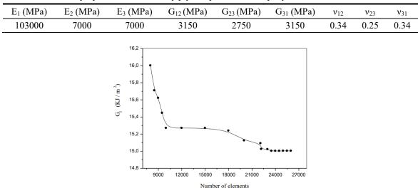
Table 1 Mechanical properties for elementary ply composite carbon/epoxy
