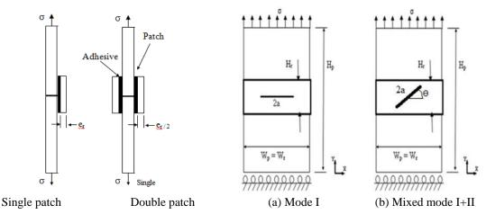
Fig. 1 Geometric model of plate with single and double patch for the pure mode I and mixed mode I+II
