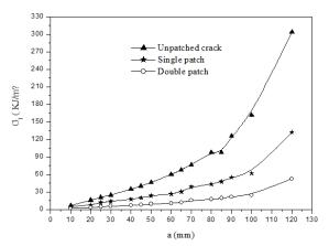
Fig. 8 Comparison of the fracture energy between patched and unpatched cracks
