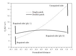
Fig. 9 Variation of the fracture energy GI along the crack front
