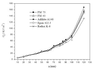
Fig. 11 GI vs crack length for different adhesives
