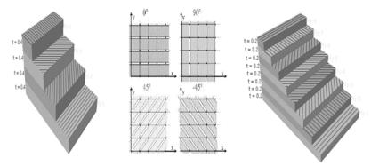
Fig. 3 Plies orientation in the patch and plate
