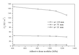
Fig. 12 Variation of the GI according to the adhesive shear modulus
