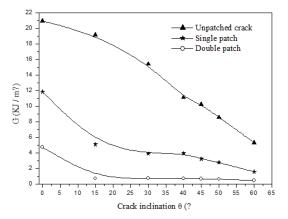
Fig. 16 Comparison of the fracture energy between patched and unpatched cracks in mixed mode
