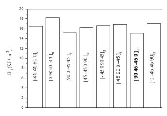
Fig. 6 Effect of plies orientation of the repaired plate on the GI values
