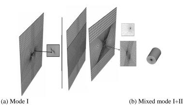
Fig. 2 Typical mesh model of the plate, patch and near the crack tip in pure mode I and mixed mode I+II
