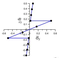
Fig. 10 Through-the-thickness variation of in-plane normal stress  $(\bar{\sigma}_y)$  for three layered  $(0^{\circ}/90^{\circ}/0^{\circ})$  symmetric laminated composite square plate (S=4)
