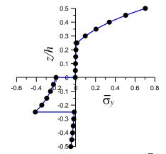
Fig. 7 Through-the-thickness variation of in-plane normal stress  $(\bar{\sigma}_y)$  for four layered  $(0^{\circ}/90^{\circ}/0^{\circ}/90^{\circ})$  antisymmetric laminated composite square plate (S=4)
