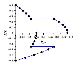
Fig. 8 Through-the-thickness variation of transverse shear stress  $(\overline{\tau}_{xz})$  for four layered  $(0^{\circ}/90^{\circ}/0^{\circ}/90^{\circ})$  antisymmetric laminated composite square plate (S=4)
