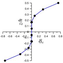
Fig. 9 Through-the-thickness variation of in-plane normal stress ( $\bar{\sigma}_x$ ) for three layered (0°/90°/0°) symmetric laminated composite square plate (S=4)
