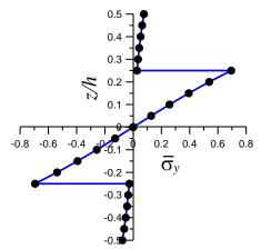
Fig. 13 Through-the-thickness variation of in-plane normal stress  $(\bar{\sigma}_y)$  for four layered  $(0^{\circ}/90^{\circ}/0^{\circ})$  symmetric laminated composite square plate (S=4)
