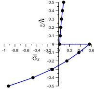
Fig. 4 Through-the-thickness variation of in-plane normal stress  $(\overline{\sigma}_x)$  for two layered  $(0^{\circ}/90^{\circ})$  antisymmetric laminated composite square plate (S=4)
