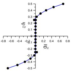
Fig. 12 Through-the-thickness variation of in-plane normal stress  $(\bar{\sigma}_x)$  for four layered  $(0^{\circ}/90^{\circ}/90^{\circ}/0^{\circ})$  symmetric laminated composite square plate (S=4)
