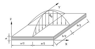
Fig. 3 Laminated composite plate subjected to sinusoidal load
