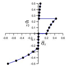
Fig. 6 Through-the-thickness variation of in-plane normal stress  $(\bar{\sigma}_x)$  for four layered  $(0^{\circ}/90^{\circ}/0^{\circ}/90^{\circ})$  antisymmetric laminated composite square plate (S=4)
