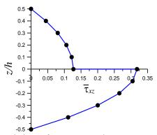
Fig. 5 Through-the-thickness variation of transverse shear stress  $(\overline{\tau}_{xz})$  for two layered (0°/90°) antisymmetric laminated composite square plate (S=4)
