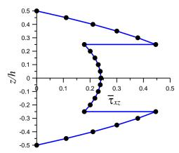
Fig. 14 Through-the-thickness variation of transverse shear stress  $(\overline{\tau}_{xz})$  for four layered  $(0^{\circ}/90^{\circ}/0^{\circ})$  symmetric laminated composite square plate (S=4)
