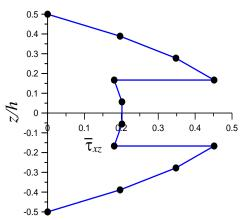
Fig. 11 Through-the-thickness variation of transverse shear stress  $(\overline{\tau}_{xz})$  for three layered  $(0^{\circ}/90^{\circ}/0^{\circ})$  symmetric laminated composite square plate (S=4)
