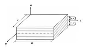
Fig. 1 Geometry and coordinate system of laminated composite plate
