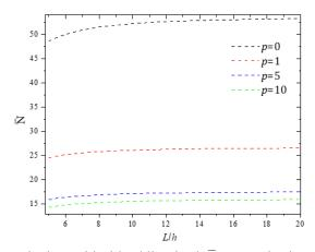
Fig. 5 Variation of the dimensionless critical buckling load  $\overline{N}$  versus slenderness ratios L/h for different values of the power law index p
