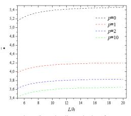
Fig. 3 Influence of the slenderness ratios L/h on the dimensionless frequency  $\varpi$  of FG beam with various power law index p
