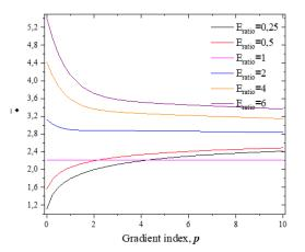
Fig. 6 Impacts of Young's modulus ratio on the dimensionless fundamental natural frequencies of S-S FG beam with respect to power-law index (L/h = 5)
