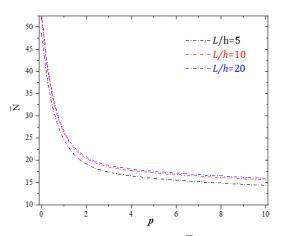
Fig. 4 Variation of the dimensionless critical buckling load  $\overline{N}$  with respect to the power law index p for different values of slenderness ratios L/h
