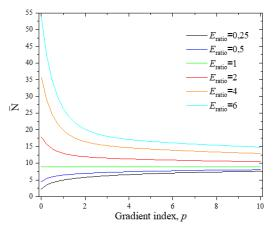
Fig. 7 Impacts of Young's modulus ratio on the dimensionless buckling loads of S-S FG beam with respect to power-law index (L/h = 5)
