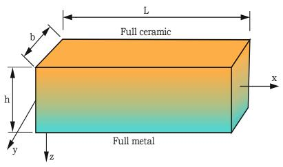
Fig. 1 Schematic arrangement of axially loaded functionally graded beam
