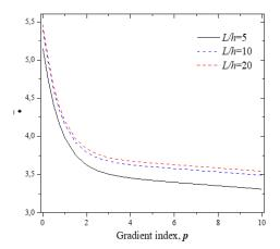
Fig. 2 Influence of the power law index p on the dimensionless frequency  $\varpi$  of FG beam with various Length to thickness ratio L/h
